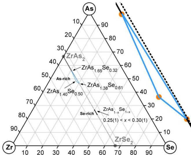
Figure S1. **Isothermal section of the ternary system Zr–As–Se at 1223 K.** The homogeneity range of the PbFCl type ternary phase is enlarged, with the dashed line indicating the tie-line between the binary compounds  $\text{ZrAs}_2$  and  $\text{ZrSe}_2$  [S2].
