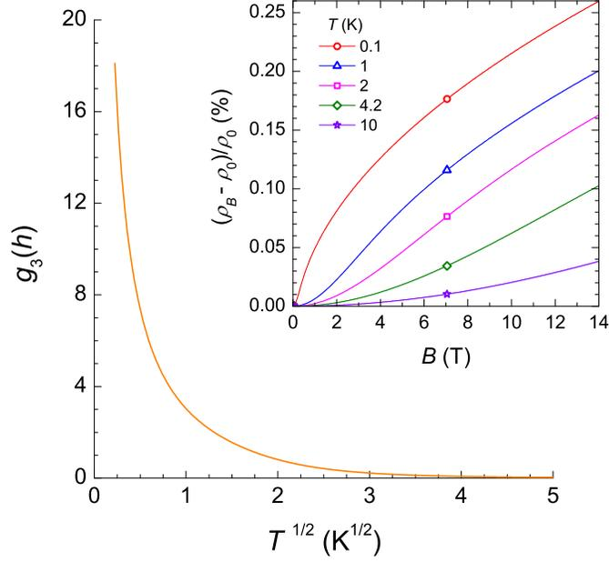
Figure S3. **Temperature dependence of the  $g_3(h)$  function.** Calculations, presented on a  $T^{1/2}$  scale, were done for the constant field  $B = 14$  T. Inset: The diffusion-channel contribution to the magnetoresistivity for various temperatures.  $D = 0.91 \text{ cm}^2\text{s}^{-1}$ ,  $\rho = 550 \mu\Omega \text{ cm}$ ,  $\tilde{F}_\sigma = 0.72$ ,  $g = 2$ .
