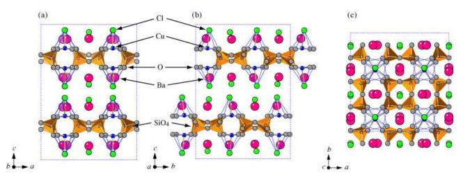
FIG. 1: (Color online) Crystal structure of  $Ba_2CuSi_2O_6Cl_2$  viewed along the (a) b axis, (b) a axis and (c) c axis.
