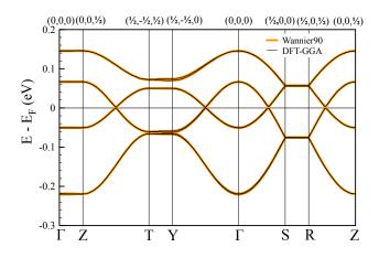
FIG. 5: (color online) Detail of the  $\operatorname{Cu-3d}_{x^2-y^2}$  band manifold around the Fermi level in  $\operatorname{Ba}_2\operatorname{CuSi}_2\operatorname{O}_6\operatorname{Cl}_2$  calculated using paramagnetic GGA-PBE and interpolated with MLWFs.
