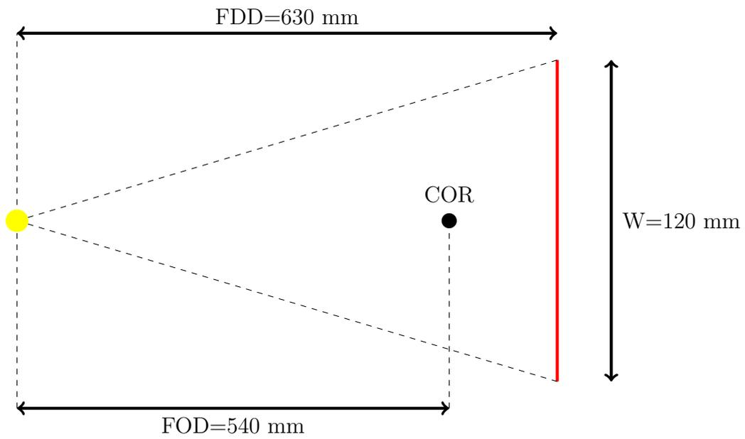
Figure 3: Geometry of the measurement setup. Here FOD and FDD denote the focus-to-object distance and the focus-to-detector distance, respectively; the black dot COR is the center-of-rotation. The width of the detector (*i.e.*, the red thick line) is denoted by  $W$ . The yellow dot is the X-ray source. To increase clarity, the  $x$ -axis and  $y$ -axis in this image are not in scale.
