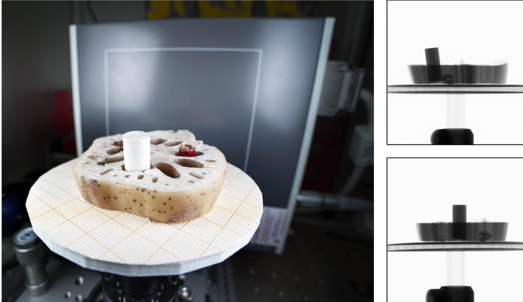
Figure 2: *Left*: Experimental setup used for collecting tomographic X-ray data. The detector plane is behind the lotus root target with the active area indicated by a white square. The target is attached to a computer-controlled rotator platform. *Right*: Two examples of the resulting 2D projection images. The fan-beam data in the sinograms consist of the (down-sampled) central rows of the 2D projection images.
