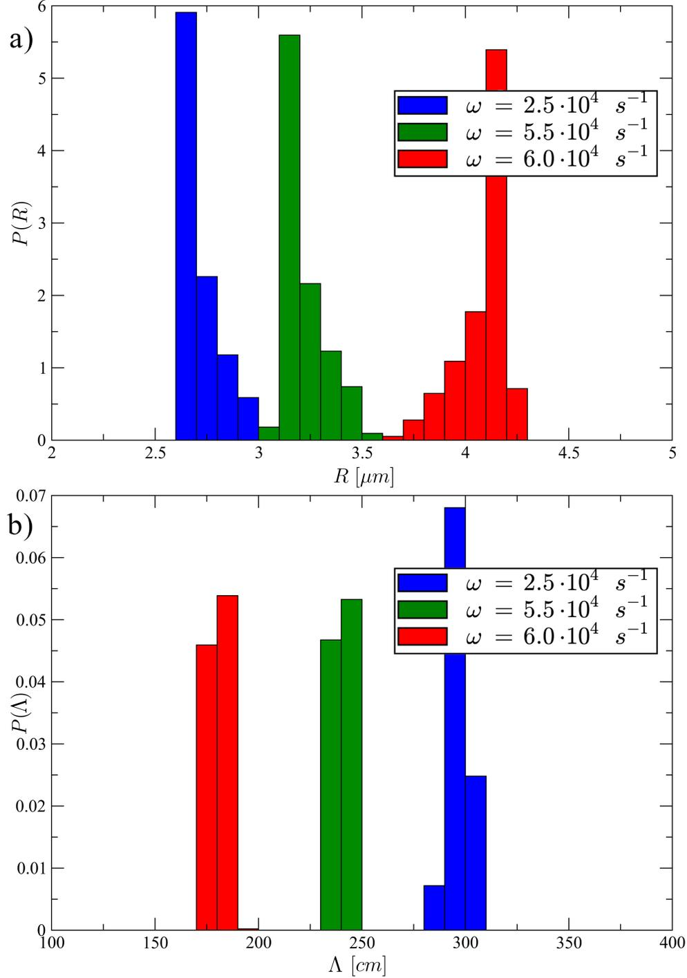
Figure 5. Top: the normalized histograms for distribution of cross section radius  $R$  at the collector for  $A = 5$  and three values of  $\omega$ . Note that the distribution of the observable during the dynamics is strongly skewed and non-gaussian. Bottom: the corresponding normalized histograms for distribution of jet path length  $\Lambda$ , showing an opposite trend with respect to  $\langle R \rangle$ .
