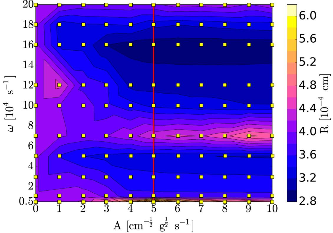
Figure 2. Contour lines showing the simulated mean jet radius  $R$  at the collector as a function of  $A \in [0, 10]$  and  $\omega \in [0.5, 20]$  parameters. The  $R(A, \omega)$  surface was assessed by a linear interpolation over a grid of pairs of  $A$  and  $\omega$ , shown in figure as yellow square symbols.
