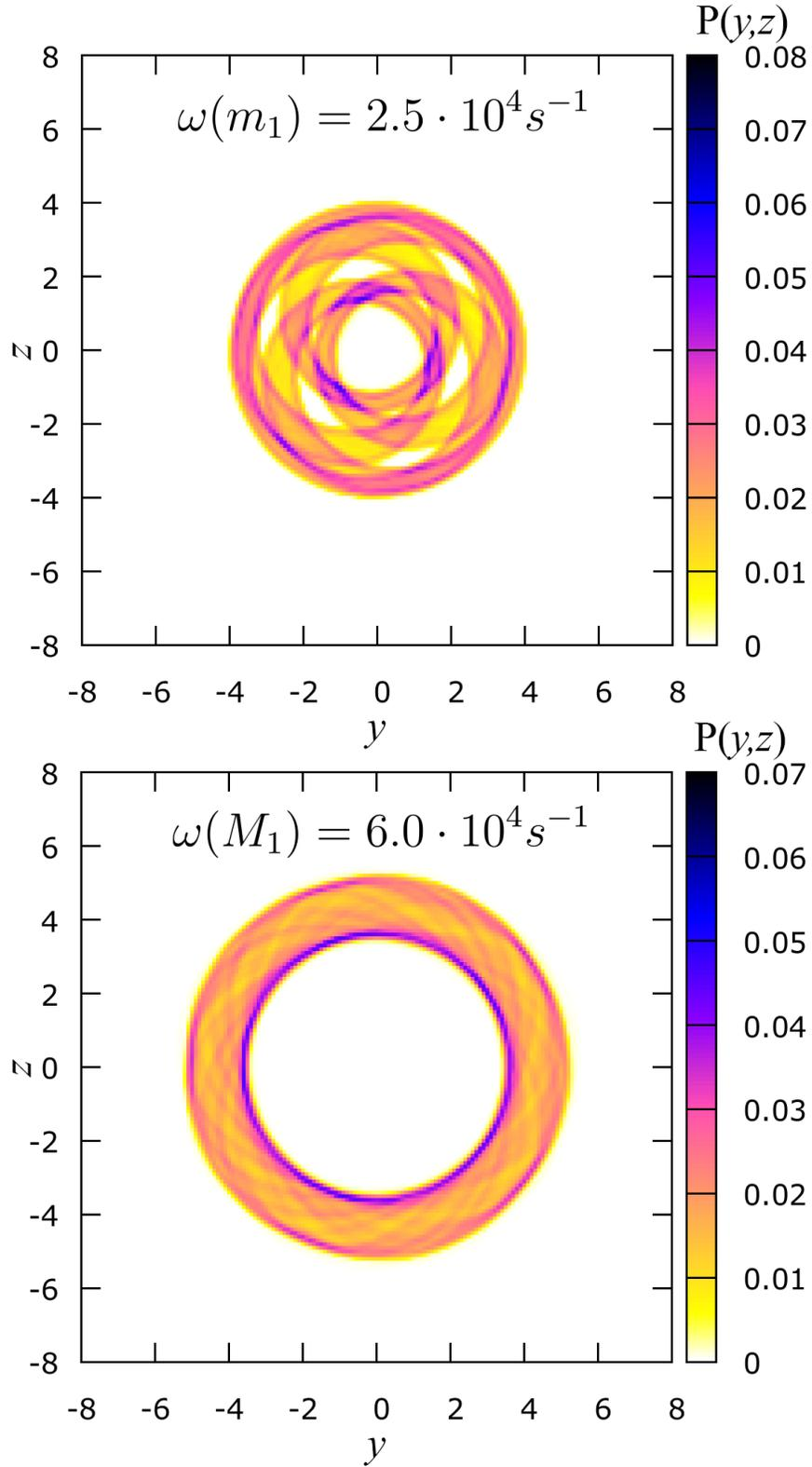
Figure 8. Normalized 2D maps computed over the coordinates  $y$  and  $z$  of the collector for the two cases with OREF at  $\omega(m_1)$  (on top panel) and  $\omega(M_1)$  (on bottom panel). The color palettes define the probability that a jet parcel hits the collector in coordinates  $y$  and  $z$ .
