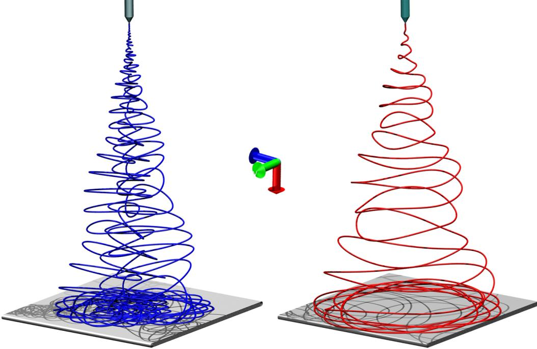
Figure 4. Jet trajectories with  $A = 5$ ,  $\omega(m_1) = 2.5 \cdot 10^4 \text{ s}^{-1}$  (left blue curve) and  $\omega(M_1) = 6 \cdot 10^4 \text{ s}^{-1}$  (right red curve). Axis convention, shown in the center, is as follows: red for  $x$  axis, green for  $y$  axis and blue for  $z$  axis. While the red curve is wider than the blue one, the latter appears more twisted, thus producing a thinner  $R$  (cfr with fig. 2 and 3).
