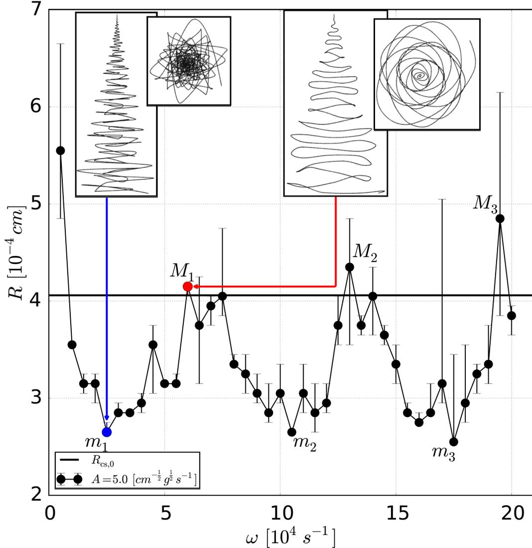
Figure 3. Mean of cross section radius  $R$  at the collector for  $A = 5$  at several values of  $\omega$ , plotted with their respective interquartile as confidence intervals. The thick solid black horizontal line represents  $R_0$ , i.e. the mean value of  $R$  in a standard electrospinning process (without OREF). The first minimum and maximum of  $R$  are highlighted in red, with the insets showing the trajectories from the lateral and bottom planes.
