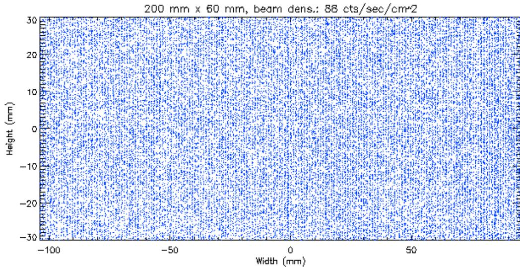
Fig. 15: final positions of the diffracted rays over a plane at a 12 m distance (the focal length of ATHENA) away from the asymmetric crystal.  $10^6$  rays were launched, 5% of them have reached the target (Fig. 14). Without a focusing module, the  $200 \times 60$  mm area is covered uniformly: the expected beam density is  $\sim 90$  ph/sec/cm<sup>2</sup> if the source monochromatic radiance is (conservatively) assumed to be  $10^{10}$  ph/sec/sterad.
