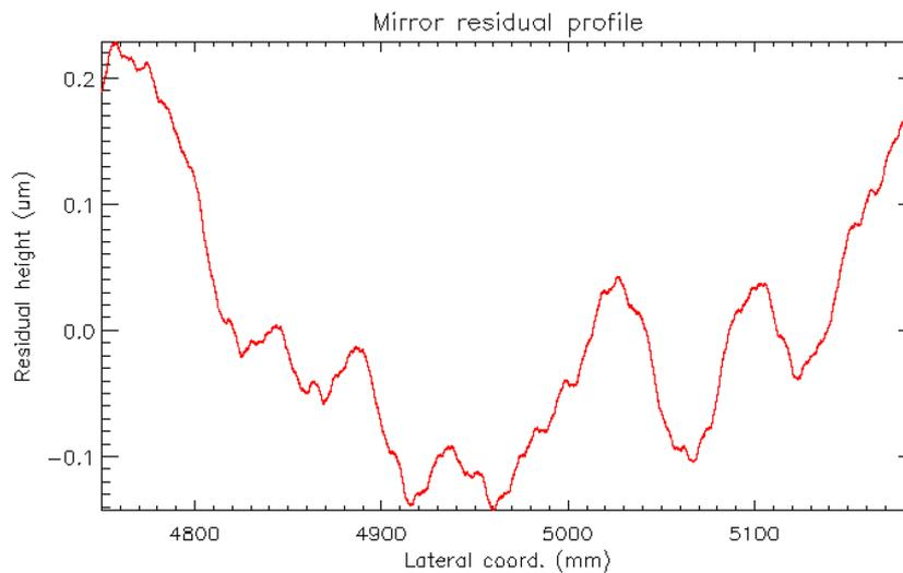
Fig. 8: one of the possible profile errors, obtained adding up 16 harmonics with constant amplitude/period ratio of 1  $\mu$ rad. This profile error gives us an idea of the tolerable figure error on the longitudinal profile of the mirror.
