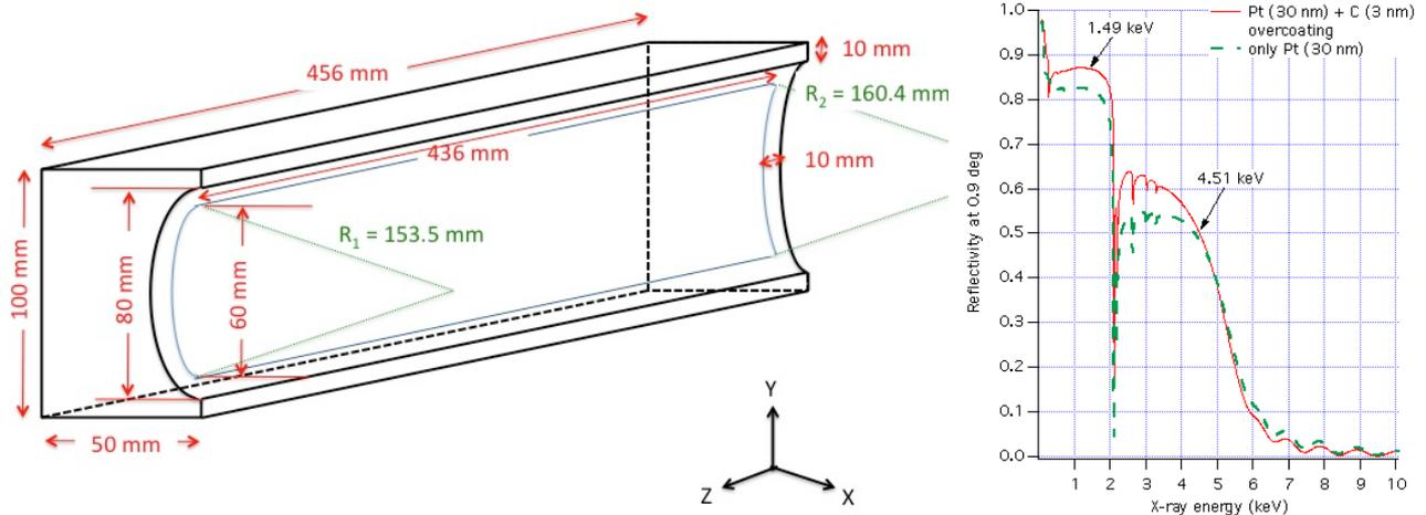
Fig. 2: (left) a drawing of the paraboloidal mirror. The focus is located 4750 mm from the mirror end with smaller curvature radius, in the direction of the positive  $z$  axis. (right) calculated mirror reflectivity.
