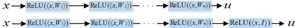
Figure 3: A network can have layers added to it without losing performance. Initially, a network has m ReLU layers with parameters \{W_1, \dots, W_m\} . A new, (m + 1) -th layer is added with W_{m+1} = I . This new layer will perform an identity mapping, therefore the two models are equivalent.
