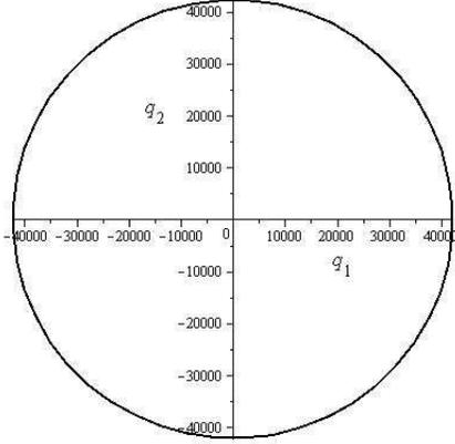
Fig. 5.— *Raduga-1M 2* satellite motion using the zonal potential  $U$ ,  $r = \sqrt{q_1^2 + q_2^2}$
