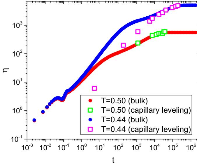
Figure 5: Bulk viscosity  $\eta$  of the polymer (filled circles) as a function of time, extracted via eqs.3 by integrating the merged data for  $G(t)$  obtained from the MD simulations and the Rouse model approximation. The open squares represent the capillary-leveling results for  $\eta_{film}(t)$  listed in table 1.
