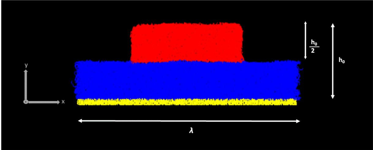
Figure 8: Polymer film with a square surface profile (periodic boundary conditions in the horizontal directions) placed here on an explicit substrate and bearing a total number of  $n = 3456$  chains with  $N = 16$  monomers each, after the heating ramp to  $T = 0.44$ . (colour code: red = top layer, blue = bottom layer, yellow = substrate).
