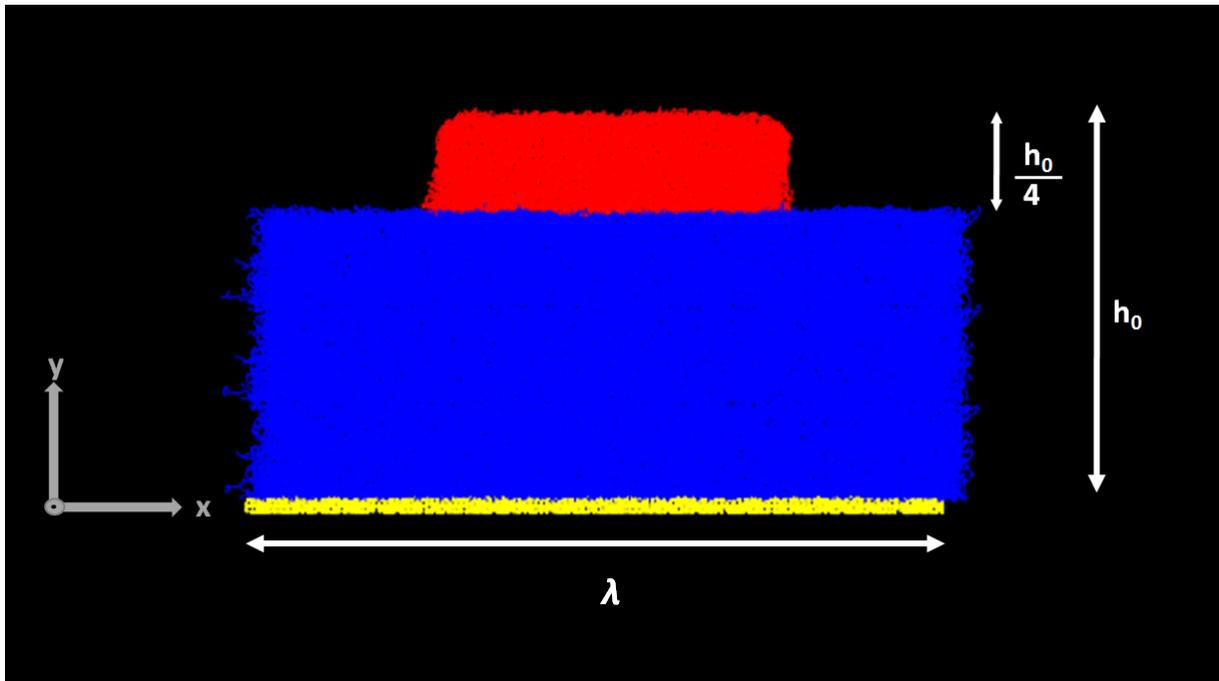
Figure 2: Configuration of the polymer-film model bearing a total number of  $n = 8064$  chains with  $N = 16$  monomers each, after the heating ramp to  $T = 0.44$ . Periodic boundary conditions are applied in the horizontal  $x, z$  directions.  $\lambda = 2B_x$  stands for the horizontal wavelength, i.e. the  $x$ -dimension of the simulation box and  $h_0$  is the maximum vertical height (colour code : red = top layer, blue = bottom layer, yellow = substrate).
