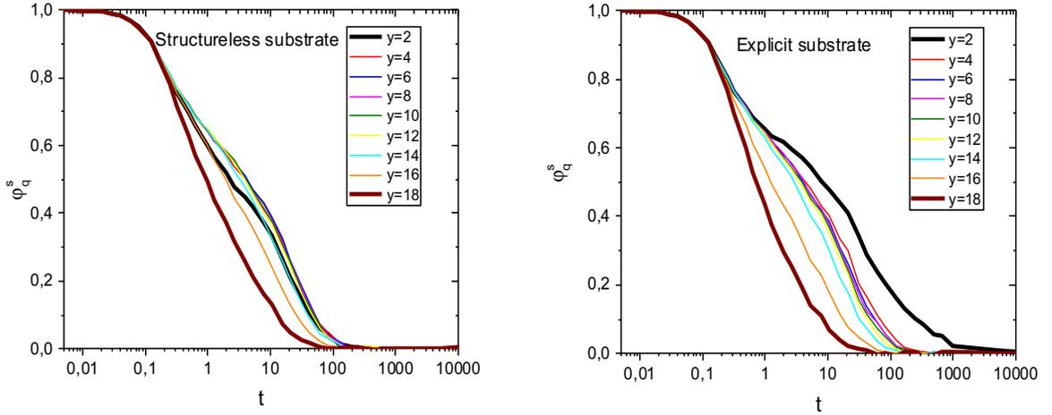
Figure 7: Layer-resolved incoherent scattering function at  $q = 6.9$  (corresponding to the maximum of  $S(q)$ ) and  $T = 0.50$ , with  $y$  being the distance from the wall represented either implicitly (left) or by explicit substrate particles (right).
