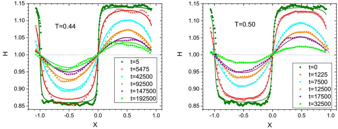
Figure 4: MD height profiles (symbols) at different times as indicated, for two temperatures:  $T = 0.44$  (left) and  $T = 0.50$  (right). The solid lines are fits to eq.7 with the dimensionless times  $T^*$  as free parameters (see table 1).  $X = 0$  corresponds to the position of the left side of the square pattern.
