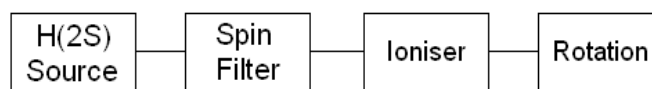
Figure G.7. Schematic diagram showing the major components of the Lamb-shift polarized ion source. H(2S) Source – a source of the metastable hydrogen (of deuterium) atoms; Spin Filter – a system of fine-tuned static magnetic, electric, and RF fields producing hydrogen (or deuterium) atoms with aligned nuclear spins; Ioniser – a selective ioniser producing positive or negative hydrogen (or deuterium) projectiles; Rotation – spin rotation unit.
