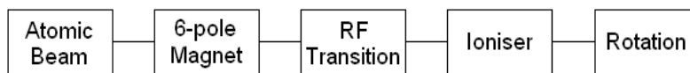
Figure G.3. A simplified schematic diagram showing the major components of the atomic beam polarized ion source. Atomic Beam – The atomic beam formation; 6-pole Magnet – An inhomogeneous magnet, sextupole or quadrupole. RF Transition – An RF unit to change the population of the hyperfine substates; Ioniser – A device used to convert the neutral atomic beam with polarized protons to negatively or positively charged ions; Rotation – A device used to change the orientation of the polarization axis.
