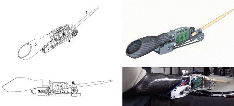
Figure 2: 1. drum stick 2. socket 3. casing for motors 4. belt connecting motor to drum stick mount 5. processor 6. drum stick mount
