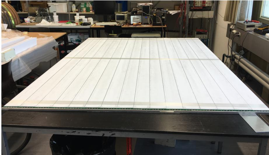
**Figure 1.** Scintillator module containing 16 scintillating strips. The external case is still to be mounted.
