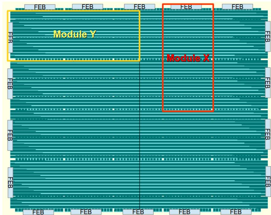
**Figure 3.** Cosmic Ray Tagger scintillator plane formed by two orthogonal layers of modules for X-Y coordinate reconstruction.
