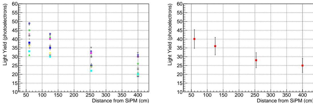
**Figure 6.** Scintillator strip response to a traversing relativistic muon as a function of distance from the readout end. Left: responses of individual strips. Right: mean and RMS of the data spread at each point.
