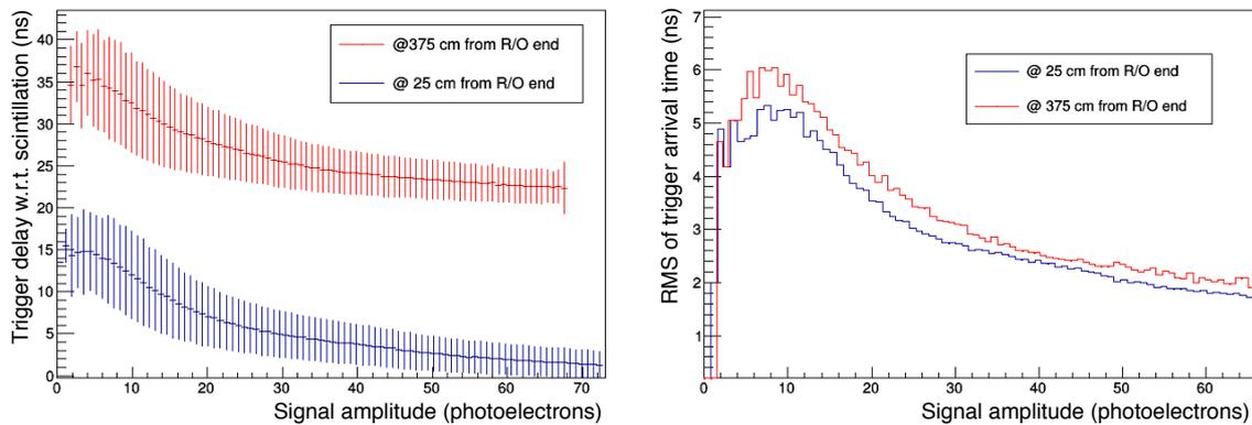
**Figure 9.** Arrival time (left) and its uncertainty (right) for the photons in CRT scintillator strips as a function of signal amplitude at a threshold of 2.5 photoelectrons. The effective photon propagation delay is  $6.1 \pm 0.7$  ns/m.
