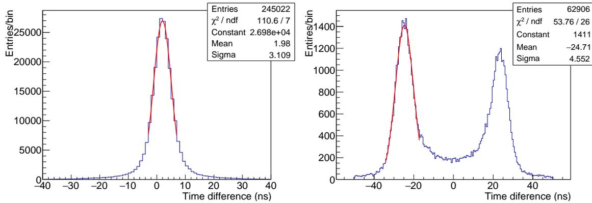
**Figure 10.** Trigger time difference distributions for two modules configuration with 0 cm (left) and 7.3 m (right) distance separation between them. Mean values correspond with delays introduced by the length of cabling used in each setup, 2 ns and 25 ns. The sigma values correspond to the trigger time resolution.
