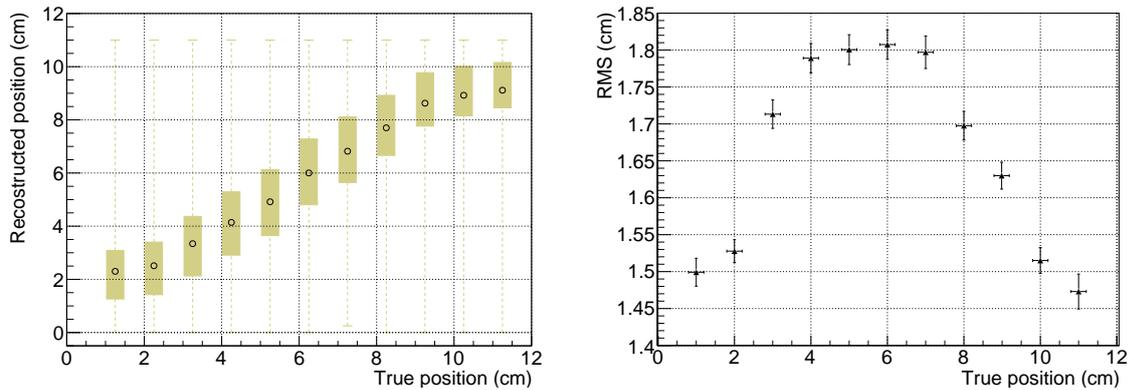
**Figure 11.** Left: position of hit derived as the weighted average of signals from left and right SiPMs. Right: RMS of the difference between the derived coordinate and the true one. The derived coordinate is corrected using the dependence in the left plot.
