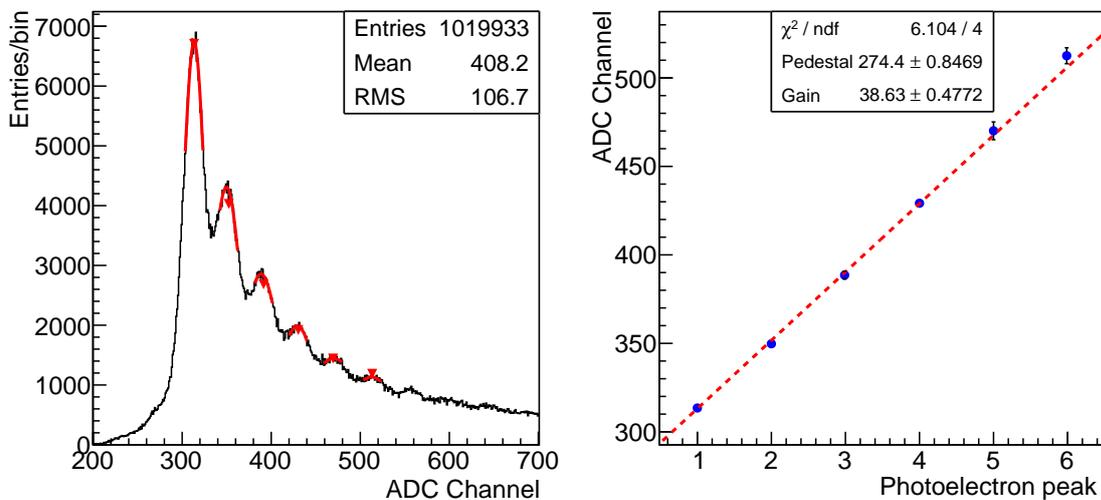
**Figure 5.** Left: SiPM spectrum obtained with ambient gamma rays. Individual photoelectron peaks are fitted to a Gaussian. Right: number of ADC counts produced by different number of photoelectrons, a linear fit allows to obtain the conversion gain factor.
