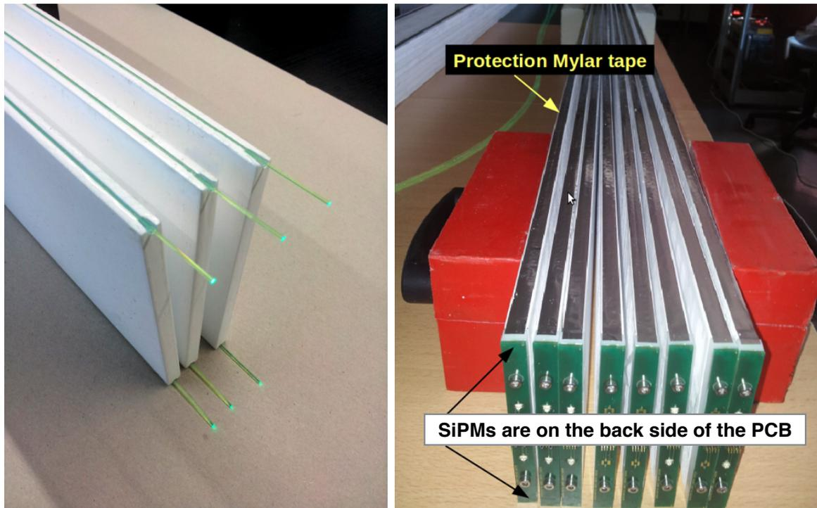
**Figure 2.** Scintillator strips with wavelength shifter fibers glued into grooves along the strip long edges. The strip is covered by a high-reflectivity white layer. The scintillation light is collected by Kuraray Y-11 wavelength shifting fibers and transmitted to the strip end where it is detected by Hamamatsu S12825-050P SiPMs.
