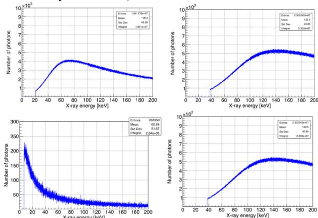
Figure 7: GEANT4 simulations of BS spectra of the 4 most common FAST beamline materials: 2 mm stainless steel (top left), 5 mm Cu frame (top right), 0.5 mm Al foil (low left) and 3 mm Nb (low right).
