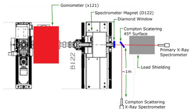
Figure 2: Forward and 90-deg (Compton scattering) detector configuration.
