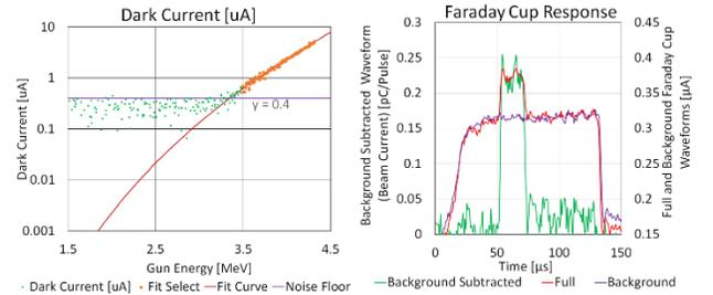
Figure 5: The gun dark current was reduced significantly by reducing the gun exit energy to  $\sim 3.5$  MeV (left). Even with the lower gun gradient, dark current from the gun dominated the overall bunch signal, as shown (right) for a 200 fC/pulse signal.
