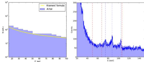
Figure 6: BS spectrum of the Al foil and its fit with Kramers's formula (right) and the sum of measured spectra for a 30 fC/pulse electron beam. Red dashed lines correspond to predicted channeling lines.
