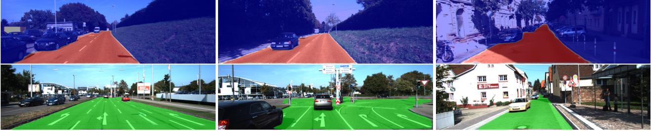
Figure 4: Visualization of the segmentation output. Top row: Soft segmentation output as red blue plot. The intensity of the plot reflects the confidence. Bottom row hard class labels.
