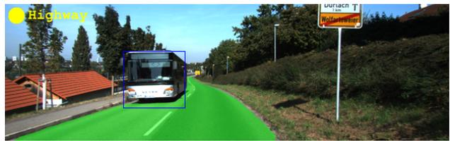
Figure 1: Our goal: Solving street classification, vehicle detection and road segmentation in one forward pass.
