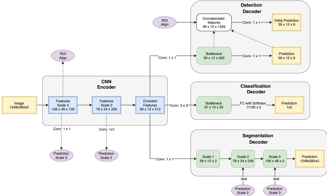
Figure 2: MultiNet architecture.
