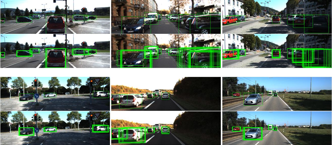
Figure 5: Visualization of the detection output. With and without non-maximal suppression applied.
