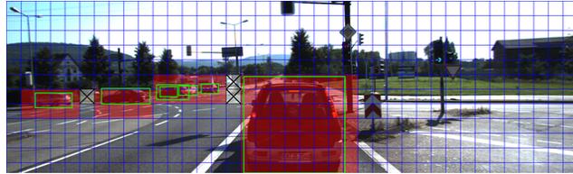
Figure 3: Visualization of our detection encoding. Blue grid: cells, Red cells: cells with positive confidence label. Transparent Cells: cells with negative confidence label. Grey cells: cells in don't care area. Green boxes: ground truth boxes.
