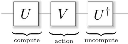
Figure 4: A compute/action/uncompute section. Since  $U^\dagger U = \mathbb{1}$ , the  $U$  and  $U^\dagger$  gate can be executed unconditionally when control qubits are added to an operation of this form. These sections can be annotated using our `Compute`, `Uncompute`, and `CustomUncompute` meta-instructions, see Sec. 4.1.3.
