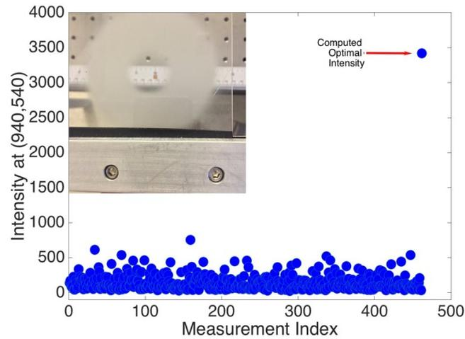
**Figure 3.** (a) groundglass sample. (b) A plot of the intensity  $|b_{(\bar{k}, \bar{l})}|$  for  $(\bar{k}, \bar{l}) = (940, 540)$  for  $\lceil M \log M \rceil \approx 461$  random trial fields (here  $M = 100$ ) followed by the intensity using the optimal wavefront  $\underline{a}_{\text{opt}}$  as in Eq. (19).
