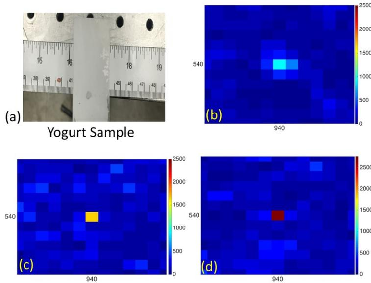
**Figure 5.** The intensity at pixels surrounding (940, 540) after a focus is generated at (940, 540) using the SDP algorithm when b)  $M = 36$ , c)  $M = 64$  and d)  $M = 100$ , respectively.
