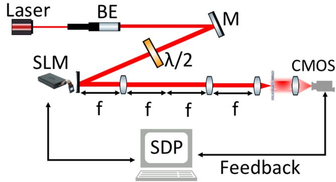
**Figure 2.** A 633 nm CW laser is expanded then spatially filtered through a lens and a  $100 \mu\text{m}$  pinhole (not shown). The polarization optics is placed before the SLM. The homogeneous beam is then reflected by the SLM that is  $4f$  imaged onto the sample. The resulting speckle pattern from the scattering sample is collected by a lens and imaged on the CMOS camera.
