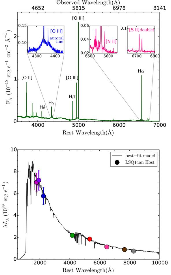
**Figure 2.** *Top:* Spectrum of the host of LSQ14an taken by VLT+X-Shooter on 2014 June 21. The spectrum in the merged data from the UVB, VIS and NIR arms, corrected to rest-frame. Host lines are labelled in the spectrum. *Bottom:* The best-fit SED of the host of LSQ14an from MAGPHYS (da Cunha, Charlot, & Elbaz 2008) shown in black line. The colour circles show photometry of LSQ14an host in the order of the Swift  $uvw2$ ,  $uvm2$ ,  $uvw1$  and Pan-STARRS1  $grizy$  filters.
