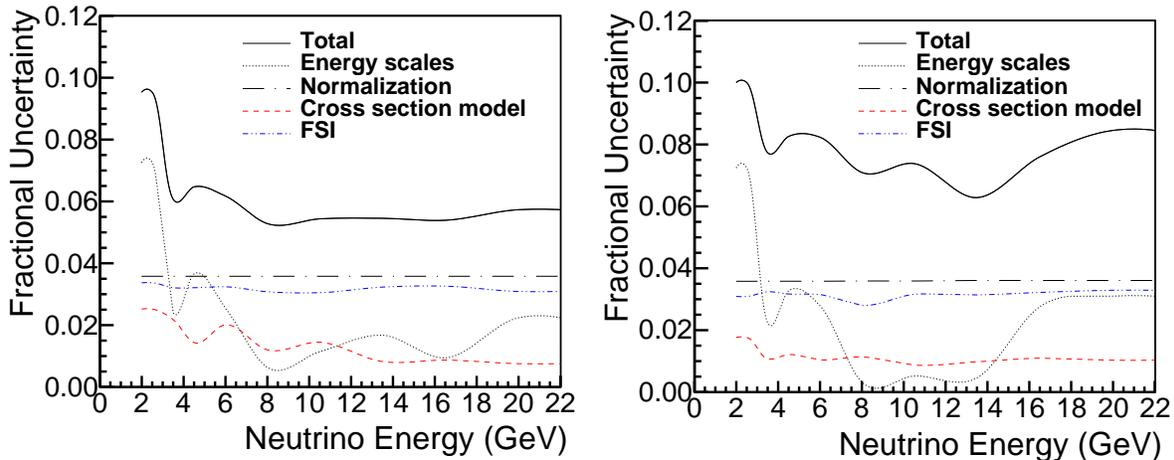
FIG. 5: Measurement uncertainties for neutrino (left) and antineutrino (right) low- $\nu$  fluxes. The total uncertainty (sys. + stat.) is the solid line. Components from cross section model (dashed red), FSI (dot-dash blue), and energy scales (dotted) are shown. The 3.6% uncertainty in the external normalization (dashed black) is the error of the NOMAD data in the normalization region.
