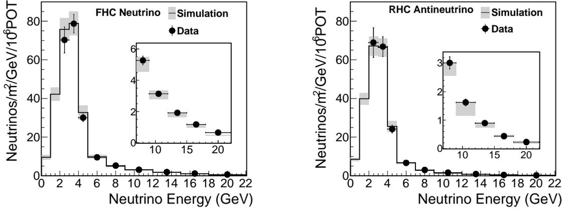
FIG. 8: Extracted low- $\nu$  flux (points) for FHC neutrino (left) and RHC antineutrino (right). The histogram shows the Monte Carlo simulated fluxes from Ref. [17] and one sigma error band (shaded bars). The insets show a zoom-in of the 7-22 GeV energy range.
