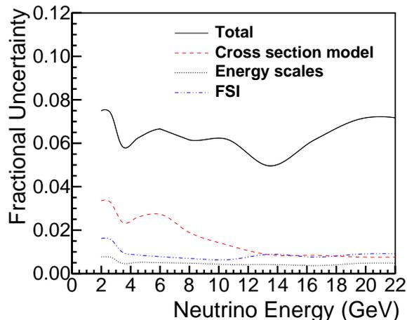
FIG. 7: Measurement uncertainties for the cross section ratio,  $R_{CC}$ . The total uncertainty (sys. + stat.) is the solid line. Components from cross section model (dashed red), FSI (dot-dash blue), and energy scales (dotted) are shown. Normalization uncertainty is very small ( $<1\%$ ) and is included in the total error curve. The uncertainty is dominated by the statistical precision of the antineutrino sample.
