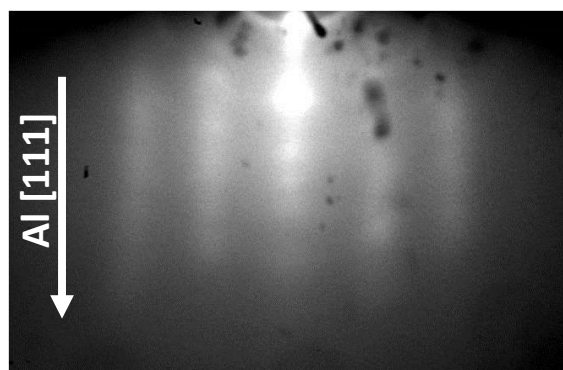
Figure S2. In situ RHEED diagram on 2.2 nm Al deposited on CVD graphene/Nickel before oxidation in ambient atmosphere.
