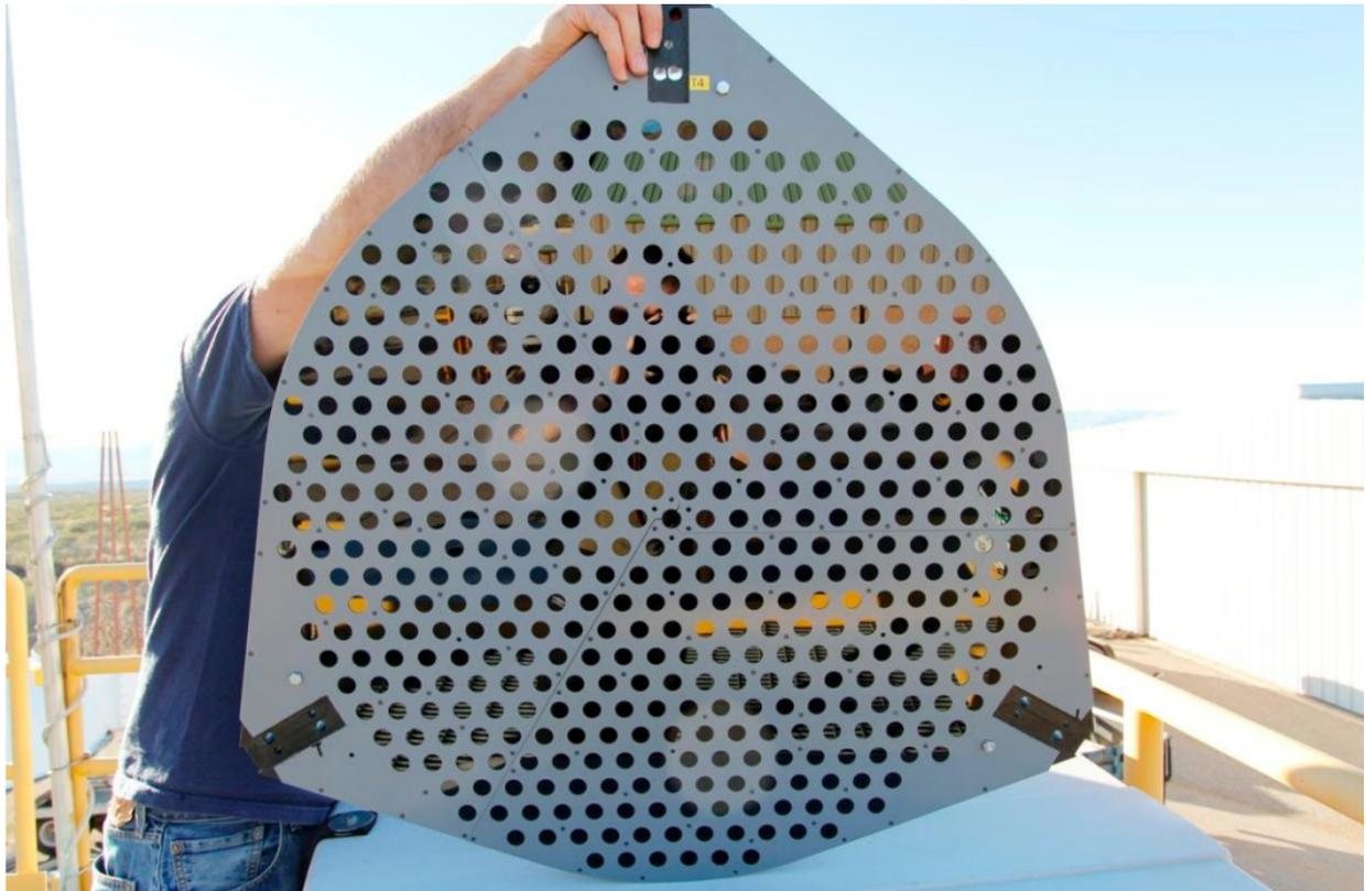
Figure 3: A UV filter plate with one filter for each PMT mounted in a central plastic layer which is then sandwiched between two thin (gray) plastic sheets with holes smaller than the filters but larger than the exit apertures of the light cones.
