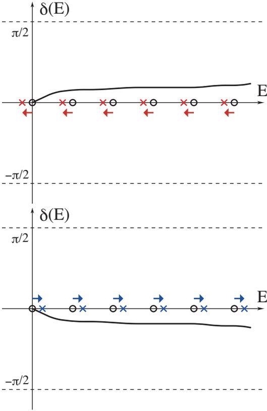
FIG. 15. Schematic illustration of the infinite-volume phase shift (solid lines), the eigenenergies of the free Hamiltonian in finite volume (circles), and the eigenenergies of the full Hamiltonian in finite volume (crosses).
