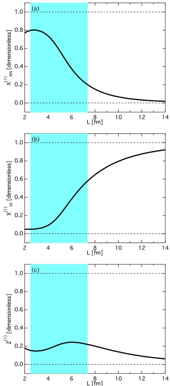
FIG. 10. Compositeness of the first excited state  $X_{\bar{K}N}^{(1)}(L)$  (a) and  $X_{\pi\Sigma}^{(1)}(L)$  (b) and the elementariness  $Z^{(1)}(L)$  (c). The shaded areas represent the region  $L_{\min} \leq L \leq L_{\max}$ .
