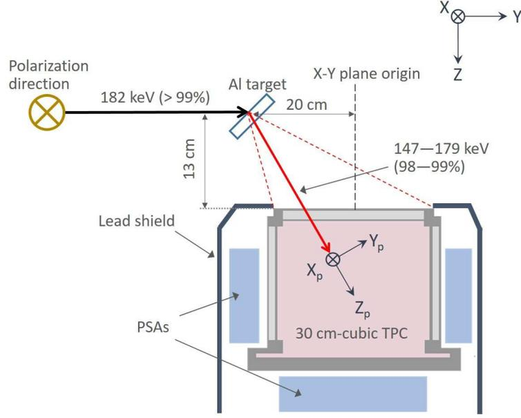
**Figure 12.** A side view in the  $Y$ - $Z$  plane of the current ETCC setup for the second experiment on BL08W at SPring-8. The  $Al$  target was shifted  $20\text{ cm}$  into the upper stream of the beamline than in the previous experiment. The photon coordinate system  $X_p Y_p Z_p$  has the  $Z$ -axis along the average direction of the incident photons, and the  $X$ -axis coincides with the  $X$ - $Y$  plane.
