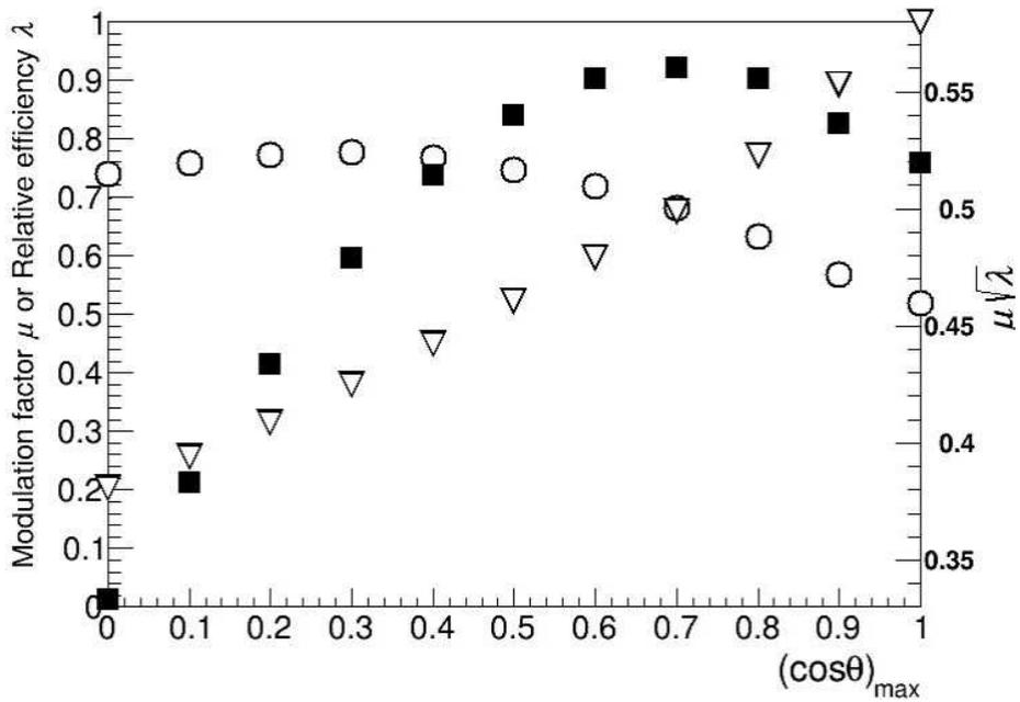
**Figure 5.** Dependences of the modulation factor  $\mu$  (open circles), the relative detection efficiency  $\lambda$  (open triangles), and the figure of merits  $\mu\sqrt{\lambda}$  (filled squares) on the integration region from 0 to  $\theta_{max}$ .
