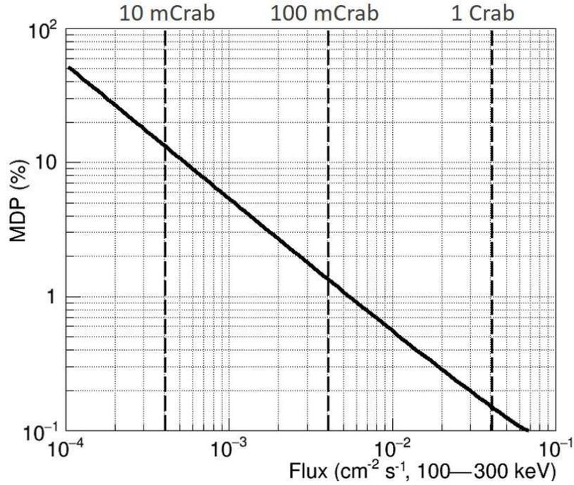
**Figure 19.** Solid line showing the calculated MDPs of the satellite-ETCC as a function of the source flux in the energy range of 100–300 keV for an observation time of  $10^7$  s. The dashed vertical lines represent source fluxes of 1, 1/10, and 1/100 the Crab nebula.
