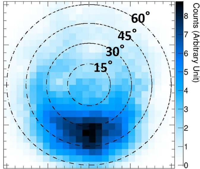
**Figure 14.** Reconstructed image showing the direction of an incident photon. The dotted concentric circles represent the incident angle ( $15^\circ$ ,  $30^\circ$ ,  $45^\circ$ , and  $60^\circ$ ) in the coordinate system of the ETCC. The spread in the image corresponds to the spread of the scattered beam. An enhancement is seen within the incident angles of  $20\text{--}40^\circ$ , and most events are concentrated near  $30^\circ$ .
