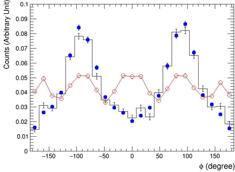
**Figure 10.** The solid line histogram represents the measured azimuthal angle distribution  $N_{pol}^{mes}(\phi)$ . The simulation results of the azimuthal angle distribution  $N_{pol}^{sim}(\phi)$  and  $N_{unpol}^{sim}(\phi)$  are plotted as filled circles and open circles, respectively.
