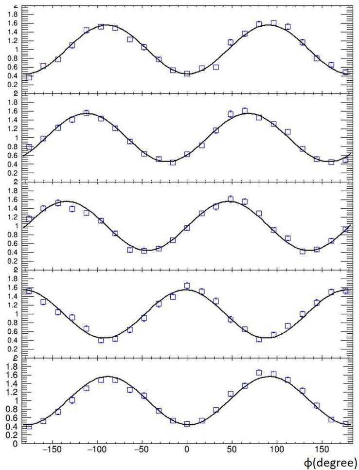
**Figure 11.** Corrected modulation curves (open squares) and the best fit curves (solid lines). The polarization direction of the X-ray beam is  $0^\circ$ ,  $-22.5^\circ$ ,  $-45^\circ$ ,  $-90^\circ$ , and  $-180^\circ$ , respectively, from top to bottom.
