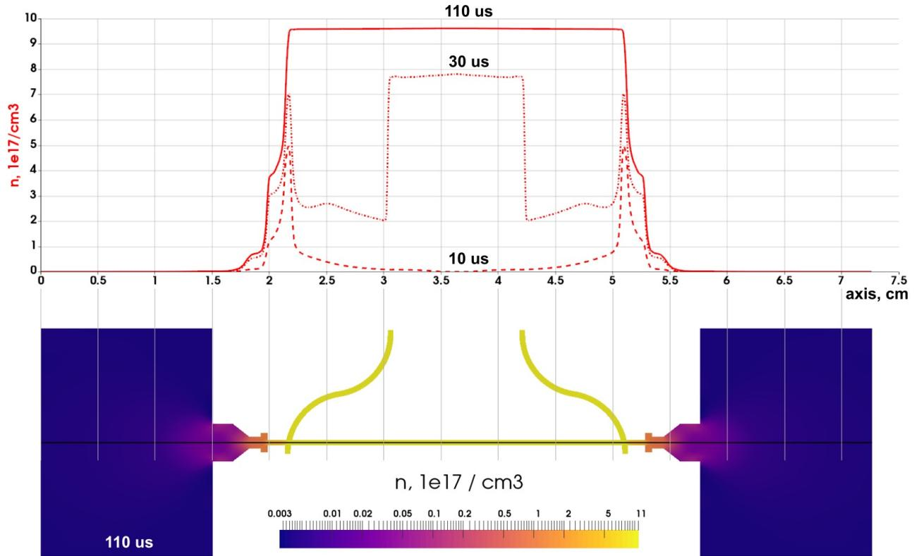
FIG. 2: On the top frame density distribution along the capillary axis (black line on the bottom frame) at the moments  $t = 10$ ,  $30$  and  $110 \mu\text{s}$  are shown. Density distribution inside the capillary and its open ends as well as in supplying channels at the moment  $t = 110 \mu\text{s}$  (steady state stage) is presented on the bottom frame.
