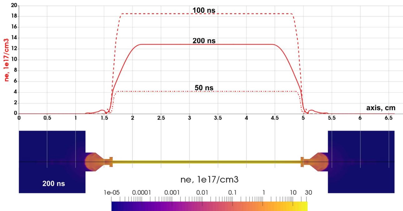
FIG. 4: Electron density distributions along capillary axis at several moments (top). Spatial distribution of electron density in the capillary and near its open ends at  $t = 200$  ns after discharge is started (bottom).
