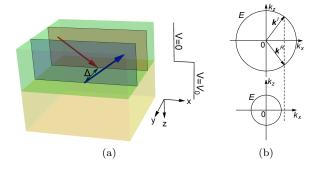
FIG. 1. (a) Schematic figure showing a light beam incident from a photonic crystal with Weyl points to another experiences a transverse shift  $\Delta$  in total reflection. (b) Schematic figure showing the condition for total reflection. The two circles represent the  $k_y=0$  cross section of the equifrequency surfaces with the same frequency E in the two photonic crystals, and  $\mathbf{k}^I$  and  $\mathbf{k}_R$  are the momentum of the incident and reflected photons, respectively.
