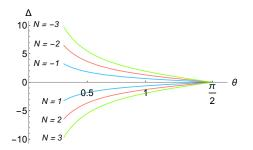
FIG. 2. Transverse shifts of a light beam during a total reflection in the interface of two photonic crystals with the same (multiple)-Weyl points.  $\theta$  is defined as  $\tan\theta \equiv k_x^I/k_z^I$ , where  $k_i^I$  is the incident momentum. Note that it is not the incident angle in general.
