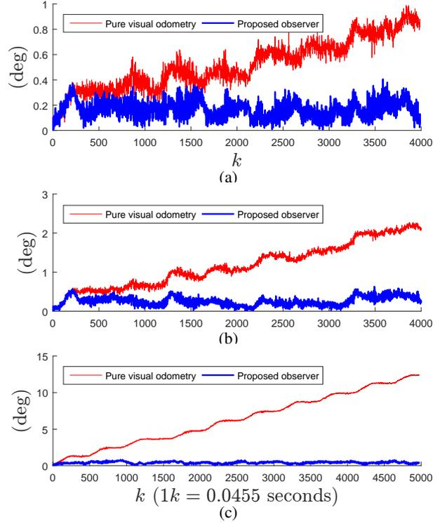
Fig. 6: Attitude estimation error of the pure visual odometry versus the proposed observer (11); (a)  $1920 \times 1200$  images are used, (b)  $960 \times 600$  images are used, (c) 1% error is added to the intrinsic camera calibration.
