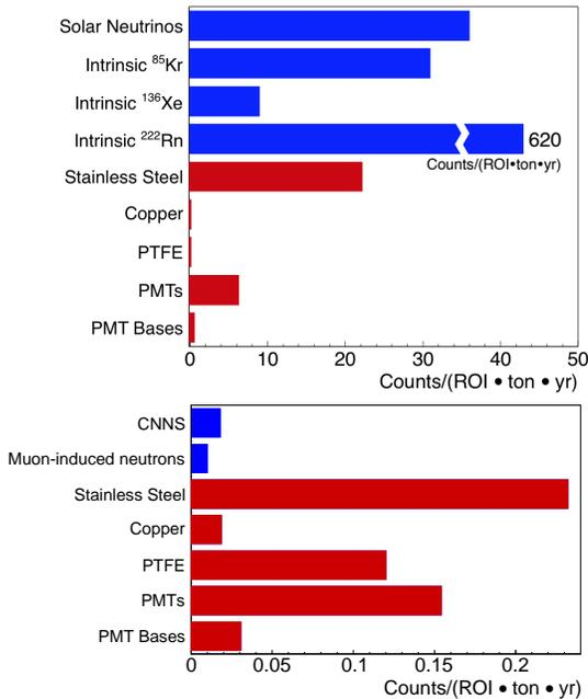
Fig. 4: Electronic recoil (top) and nuclear recoil (bottom) background contributions from materials (red) and from intrinsic and external sources (blue). The number of events per year in a 1-ton fiducial target is shown in the electron equivalent (1, 12) keV<sub>ee</sub> region of interest for electronic recoil events, corresponding to a nuclear recoil energy interval of (4, 50) keV<sub>nR</sub>.
