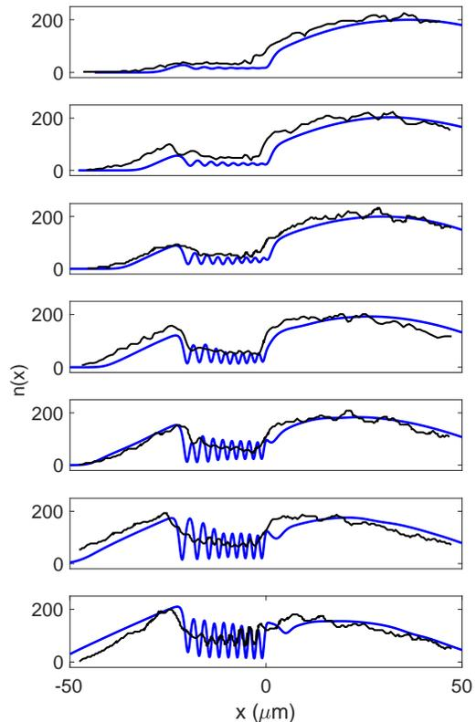
FIG. 8. The evolution of a condensate. The density profile is plotted at 20 ms intervals with moving potential step  $U_s = 0.75\mu$ , scaled by a common factor to match experiment, and viewed in the moving frame where  $x = 0$  defines the step edge. Black: experiment [3]; blue: present simulation.
