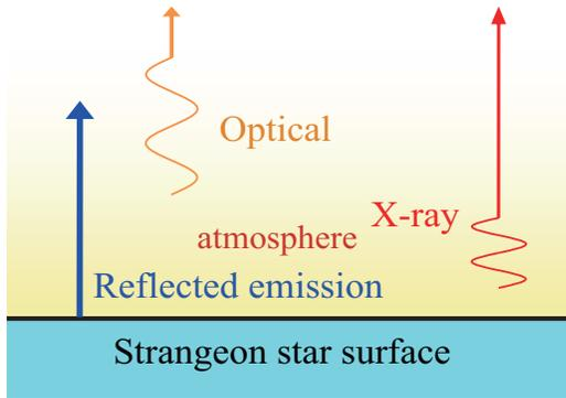
**Fig. 1** A schematic diagram of the observed radiation from the atmosphere which is on top of a strangeon star. The total observed radiation consists of the emission from the atmosphere and the reflected component by the emission-negligible surface. The radiation is optically thin at X-ray bands so that photons can emit from much deeper location, while optically thick for long wavelength photons.
