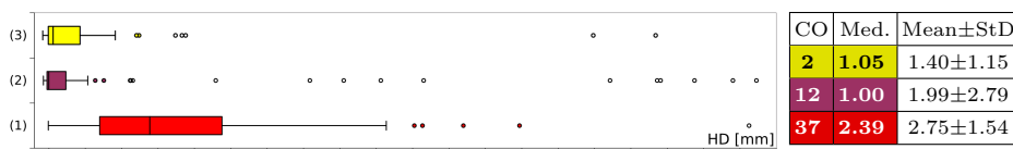
Fig. 4. Result boxplots (left) and statistics as legend (right) of the three experiments: Boxplots with Hausdorff distances (HD) [mm] and critical outliers (CO, HD > 3 mm). For experiment (2) one outlier at 18 mm is not shown in the graphics for display reasons; or overlap or are located in the maximum range (whisker).
