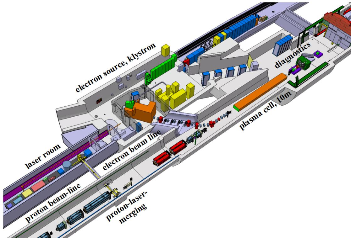
Fig. 13: Integration of the AWAKE experiment in the experimental area
