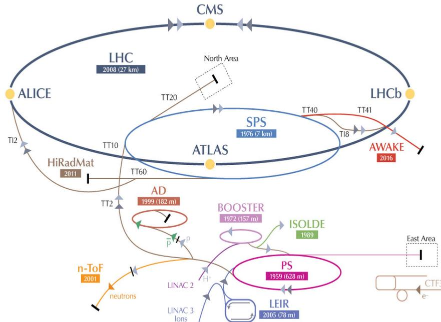
**Fig. 2:** Layout of the CERN accelerator chain
