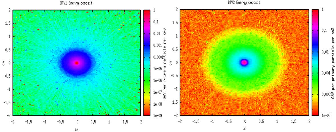
**Fig. 12:** Energy deposition in  $\text{GeV}/\text{cm}^3$  per primary proton particle of the self-modulated proton beam downstream of the plasma cell. (a) Scintillator 1 m downstream of the plasma cell. (b) Scintillator 9 m downstream of the plasma cell.
