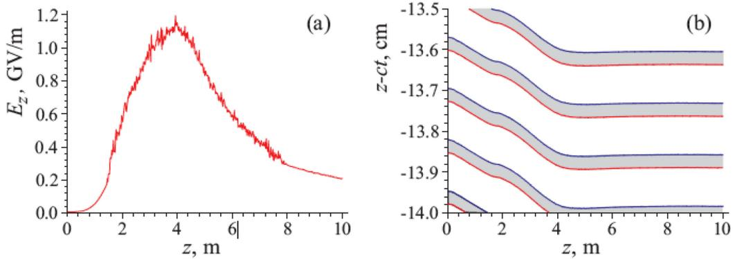
**Fig. 7:** (a) Maximum amplitude of accelerating field  $E_z$  excited along the bunch plotted as a function of position along the plasma. (b) Positions along the bunch ( $z - ct$ ) where the wakefields are both accelerating and focusing for witness electrons are shown in grey as a function of propagation along the plasma. This position varies over the first 4 m of propagation and remains at the same  $z - ct$  position after that.
