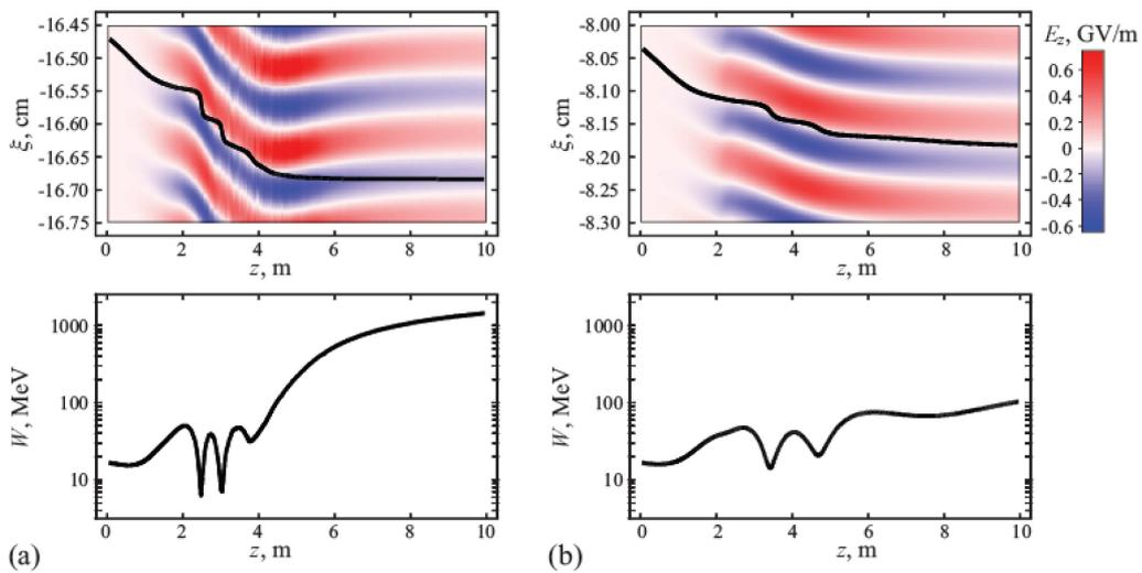
**Fig. 11:** Co-moving coordinate  $\xi$  (top) and energy (bottom) versus propagation distance for two typical test electrons injected with different delays with respect to the laser pulse. The top plot also shows the color map of the on-axis electric field  $E_z$  in the vicinity of the electron.
