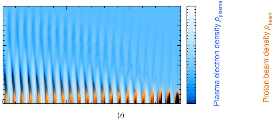
**Fig. 6:** Self-modulated proton bunch resonantly driving plasma wakefields sustained by plasma density perturbation. The plasma electron density is shown increasing from white to blue and the proton density increasing from yellow to dark red.
