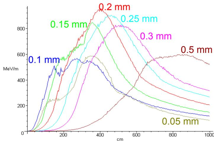
**Fig. 3:** Wakefield driven by 400 GeV proton beam along 10 m long plasma cell with different transverse beam sizes.
