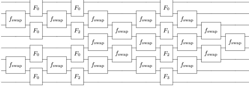
FIG. 4. Circuit to implement one-dimensional FFFT on  $M = 8$  sites, as described in [67]. Circuit is composed of  $f_{\text{swap}}$  gates and  $F_k$  gates, defined in Eq. (I16) and Eq. (I2), respectively. The circuit size is  $\mathcal{O}(M^2 \log(M))$  and its depth is  $\mathcal{O}(M \log M)$ .
