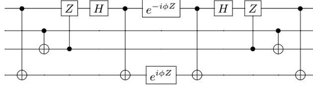
FIG. 6. Simulation circuit for  $e^{-i2\phi(a_p^\dagger a_q + a_q^\dagger a_p)}$  for use within the Trotter-Suzuki framework illustrated for  $q = p + 3$ . The analogous networks traditionally used contain 12 CNOT, 8 single qubit Clifford operations and 2 single qubit rotations and the rotations cannot be parallelized.
