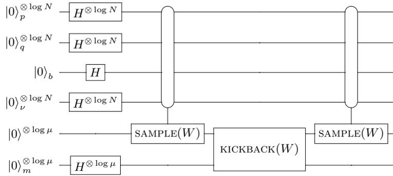
FIG. 7. The  $\text{PREPARE}(W)$  circuit. Note that the  $H$  gate is a Hadamard.  $\text{SAMPLE}(W)$  is called twice to uncompute the ancilla register. As there are only  $\mathcal{O}(\log N)$  ancilla and the gate complexities of both  $\text{SAMPLE}(W)$  and  $\text{KICKBACK}(W)$  are bounded by  $\widetilde{\mathcal{O}}(1)$ , the overall gate complexity required to implement  $\text{PREPARE}(W)$  is  $\widetilde{\mathcal{O}}(1)$  with respect to  $\epsilon$  and  $N$ .
