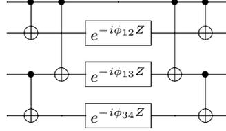
FIG. 5. Simulation circuit for  $e^{-i(Z_1 Z_2 \phi_{12} + Z_3 Z_4 \phi_{34} + Z_1 Z_3 \phi_{13})}$ . This strategy allows  $N - 1$  such terms to be simulated in parallel using a CNOT chain of depth  $\lceil \log(N) \rceil$ .
