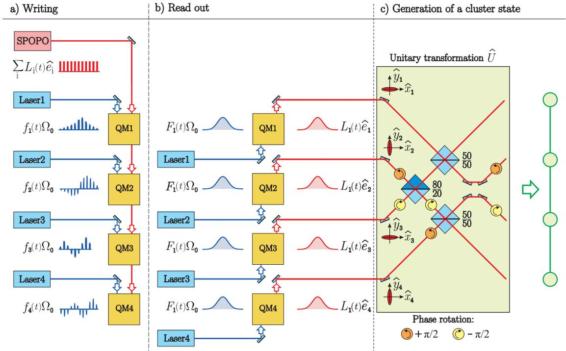
Figure 6: Scheme of the thought experiment on generation of a light linear cluster consisting of four nodes.
