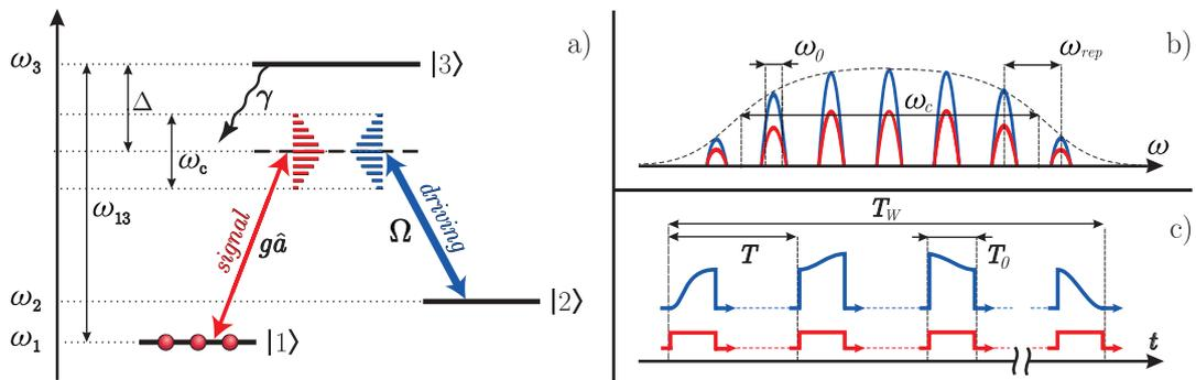
Figure 1: a) Energy level scheme of an atomic ensemble, interacting with combs of signal and driving in the Raman memory protocol; b) frequency profile of the signal and driving fields:  $\omega_c$  – spectral width of the combs,  $\omega_{rep}$  – distances between the comb’s teeth,  $\omega_0$  – width of a single tooth; c) time profile of the signal and driving fields:  $T_W$  – total duration of the periodic pulse trains,  $T$  – repetition period,  $T_0$  – duration of a single pulse.
