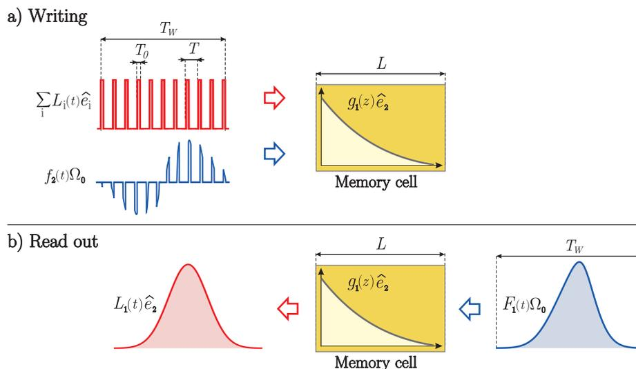
Figure 5: Schematic representation of the shape converter for the signal field.
