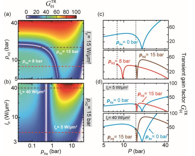
FIG. 1. Transient exponential gain factor  $G_{01}^{\text{TR}}$  plotted against (a)  $p_{\text{H}_2}$  and  $p_{\text{Xe}}$  for  $I_p = 15 \text{ W}/\mu\text{m}^2$  and (b)  $I_p$  and  $p_{\text{Xe}}$  for  $p_{\text{H}_2} = 15$  bar. (c) and (d) are cuts through at the positions of the horizontal dashed lines in (a) and (b), respectively. The blue curves in (c) and (d) show the behavior when  $p_{\text{Xe}} = 0$ .
