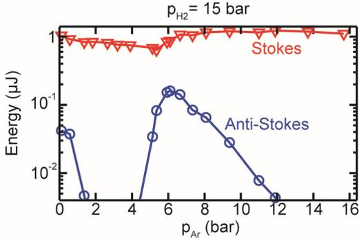
Fig. S4. Experimental (symbols) energy in the first Stokes and anti-Stokes for a pump energy of 3.60  $\mu\text{J}$  in a mixture of  $\text{H}_2$  and Ar, plotted as a function of Ar pressure at  $p_{\text{H}_2} = 15$  bar.
