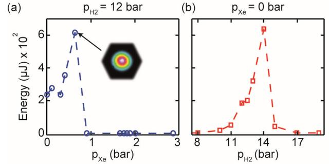
Fig. S3. Experimental (symbols) energy in the 2<sup>nd</sup> anti-Stokes sideband generated in (a) a H<sub>2</sub>-Xe mixture, plotted versus  $p_{\text{Xe}}$  when  $p_{\text{H}_2} = 12$  bar and (b) when  $p_{\text{Xe}} = 0$  bar. A near-field image taken with a CCD camera is also shown in (a). The dashed connecting lines are just intended as guides for the eye.
