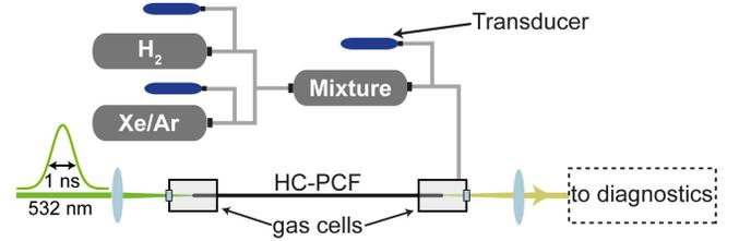
FIG. 3. Schematic diagram of the experiment. The pressure scan was performed in steps of  $\sim 100$  mbar of buffer gas. Near-field images and sideband energies were recorded at each pressure point.
