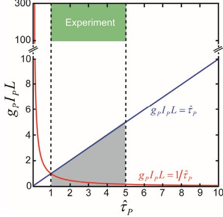
Fig. S1. The overall Raman gain plotted against  $\hat{\tau}_p$  for a pump pulse with 1 ns duration. The blue and red curves show the limits for transient and high gain operation, respectively. In the experiments  $(g_p I_p L)_{\text{Exp}} > 100$  and  $\hat{\tau}_p$  lies in the region between the dashed lines (the green shaded region). This places us in the strongly transient regime.
