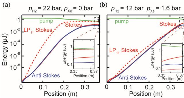
FIG. 5. Simulated evolution of the sideband energies with propagation distance at the maximum of anti-Stokes emission and 3.6  $\mu\text{J}$  pump energy for (a)  $p_{\text{H}_2} = 22$  bar and  $p_{\text{Xe}} = 0$  and (b)  $p_{\text{H}_2} = 12$  bar and  $p_{\text{Xe}} = 1.6$  bar. The parameters are otherwise identical to those in Fig. 4. The dashed red curve shows the  $\text{LP}_{11}$ -like Stokes signal, and the insets plot the evolution over the last 2 cm of fiber in both cases.
