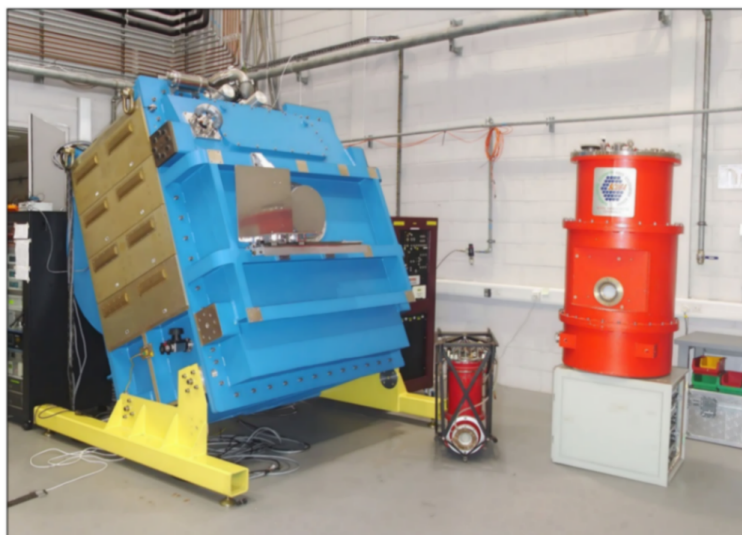
Figure 21. The JCMT continuum instruments together in the ROE Crawford laboratory, prior to the delivery of SCUBA-2 to JCMT (left) SCUBA-2 (10,000 pixels) (centre) UKT14 (1 pixel) and (right) SCUBA (128 pixels). SCUBA now resides in the National Museum of Scotland in Edinburgh. Photograph courtesy of the Royal Observatory Edinburgh.
