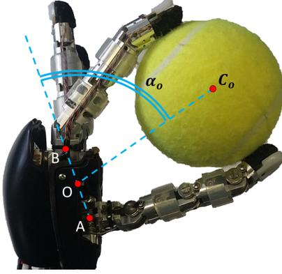
Fig. 2: The object center  $C_o$  is defined as the halfway point between the two points of contact. The object position  $\alpha_o$  is defined as the angle between the vectors  $\vec{OC}_o$  and  $\vec{OB}$ .  $A$  and  $B$  are set at the base of, respectively, the thumb and the middle finger, while  $O$  lies at middle distance between  $A$  and  $B$ .
