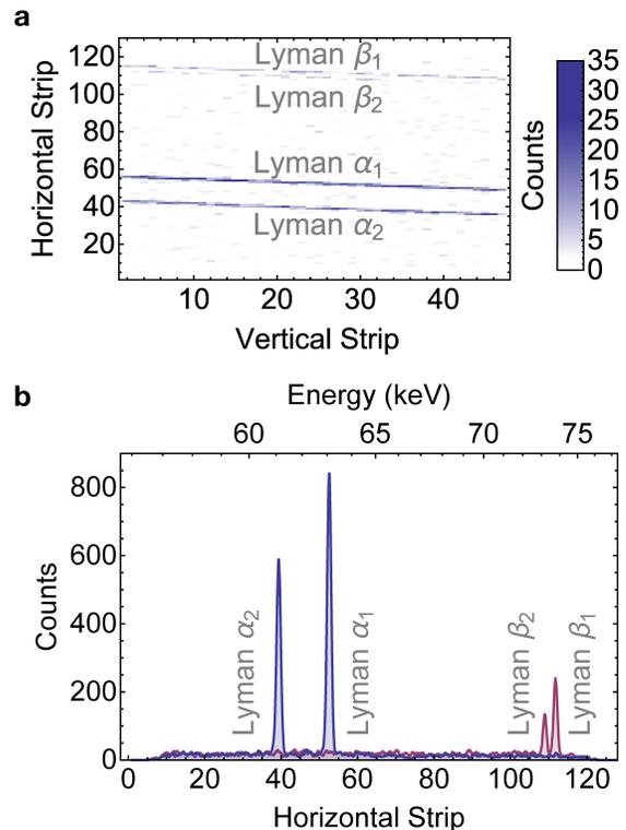
FIG. 2. (a) Coincident x-ray spectrum as recorded by one of the FOCAL spectrometers. (b) Spectrum of the Lyman- $\alpha$  and - $\beta$  doublets of  $\text{Au}^{78+}$  obtained by a projection of the respective two-dimensional intensity distribution shown in (a).
