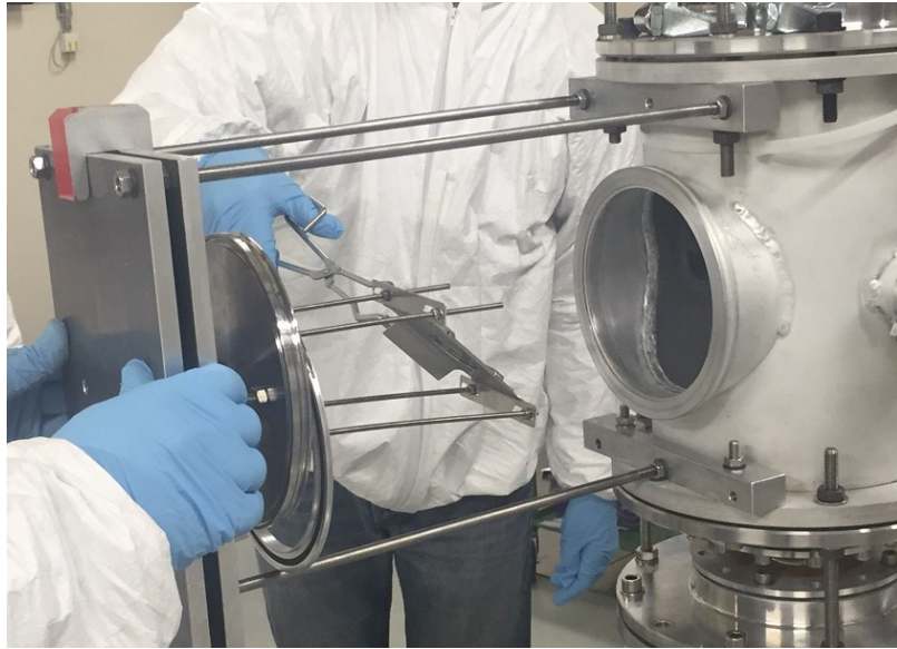
Figure 5. Insertion of the ^7\text{Be} radioactive target in the setup, with a support independent of the telescope detector installed from the opposite side of the chamber.
