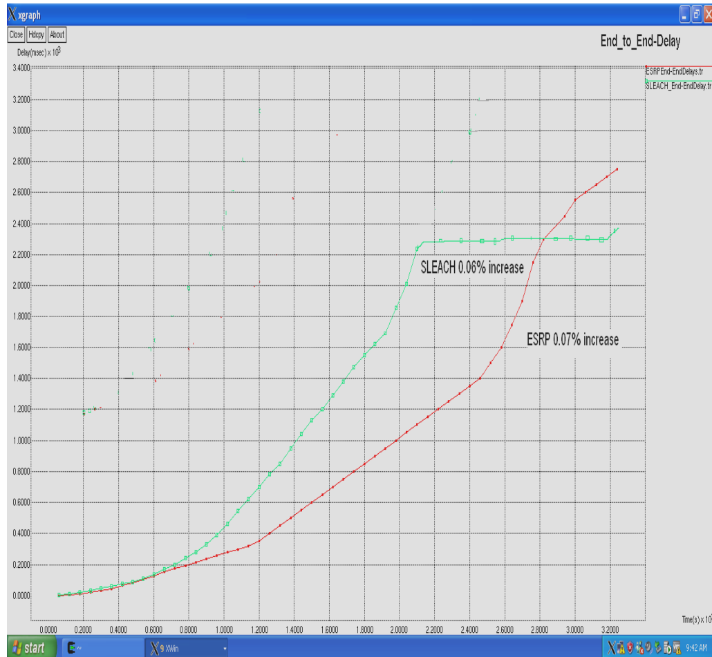
Figure 3.30 Comparison of ESRP and SLEACH in terms of ‘End to end delay’
