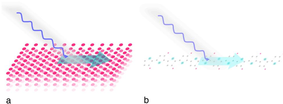
**Figure 1.** Both in surfaces of crystalline metals or semiconductors (a) and in quasi-one-dimensional molecules like polymers (b), a local coherent forcing, e.g., by a laser beam (blue wavy lines), can induce directed currents (green arrows). They combine a spatially periodic static potential, possibly asymmetric under reflection, as in ratchets, with a local periodic driving that breaks time-reversal invariance, as in pumps.
