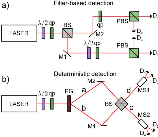
Fig. 8. A vector vortex beam is generated by transforming a linearly polarised Gaussian laser beam with a half-wave plate and a  $q$ -plate. (a) The vector beam is sent along two path, each having a vector mode filter based on geometric phase. (b) The generated vector beam is passed through a Mach-Zehnder interferometer that resolves intra-modal phases. The two outputs of the interferometer are sent to OAM mode sorters that resolves the OAM content.
