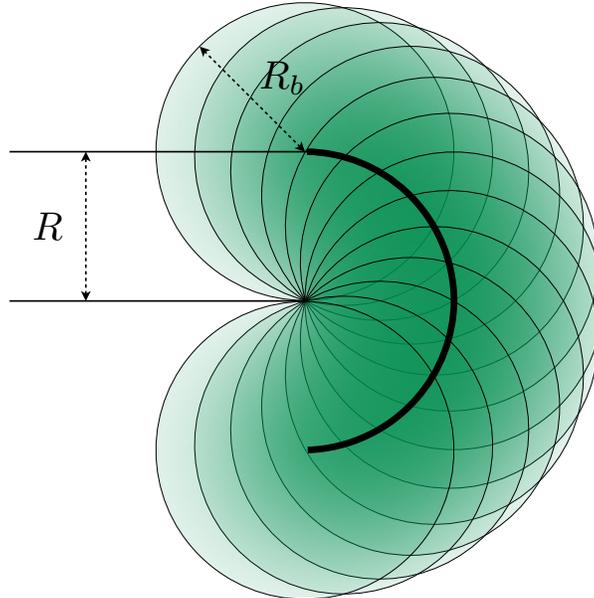
FIG. 4. An illustration of a semicircular body of radius  $R$  composed of 13 circular beads of the same radius  $R_b = R$ . The center of every bead lies on the arc of the semicircle (thick solid line), with any adjacent pair of them separated by equal angular distance.
