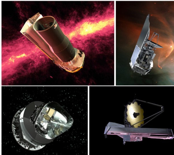
Fig 6 Four examples of satellites that observe at mid/or far-infrared wavelengths (§3). Top row : Spitzer and Herschel . Bottom row : Planck and JWST , which also use V-groove radiators (thermal shields) to achieve passive cooling to < 40 K.
