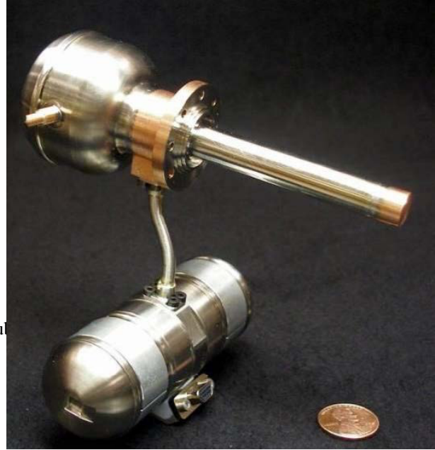
Fig 14 The Lockheed Martin Coaxial Micro Pulse Tube Cryocooler, which will provide cooling to 120 K for the CubeSat Infrared Atmospheric Sounder (CIRAS), scheduled for launch in 2019 (179) . This cooler weighs less than 0.4 kg, and has reached TRL \geq 6 .
