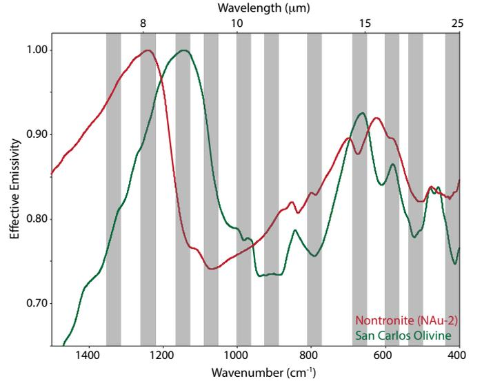
Figure 7: Two example thermal emission spectra of olivine (anhydrous silicate mineral) and nontronite (aqueously altered silicate mineral). Shaded regions indicate example spectral bands for TMC that provide compositional discrimination in addition to temperature mapping.
