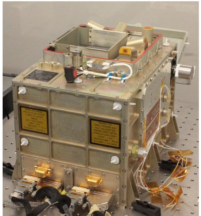
Figure 15: The GIADA spare model housed in a clean room for calibration and testing activities performed during the *Rosetta* cruise and scientific phase. On the top of the instrument the squared baffle of the dust particles that are detected first by the Grain Detection System (GDS), and then by the Impact Sensor (IS) mounted at the bottom of the instrument. The microbalances are the 5 cylinders distributed around the GIADA entrance.
