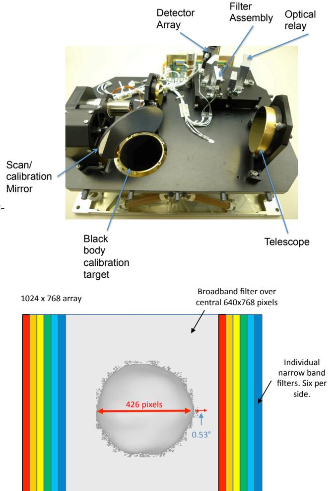
Figure 9: (Top) The TMC heritage instrument, the Compact Modular Sounder (CMS), flight unit minus its outer cover. CMS has approximate dimensions of  $380 \times 335 \times 185$  mm. (Bottom) Proposed filter and imaging detector layout, example shown during approach phase to the MBC. The TMC will use an optimised layout, reducing the instrument size to  $180 \times 150 \times 120$  mm. Mass is 4 kg based on the CMS design.
