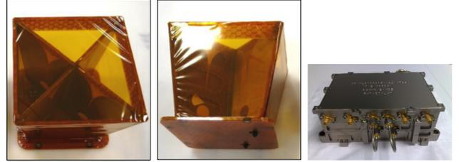
Figure 11: SSR antenna and electronics box.
