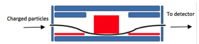
Figure 19: ChaPS Bessel box geometry. Red are the electrodes that hold the voltage and blue are at ground.
