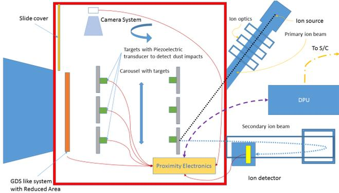
Figure 16: Schematics of DIDIMA merged dust instrument
