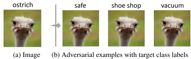
Figure 1: Visual illustration of adversarial examples crafted by EAD (Algorithm 1). The original example is an ostrich image selected from the ImageNet dataset (Figure 1 (a)). The adversarial examples in Figure 1 (b) are classified as the target class labels by the Inception-v3 model.
