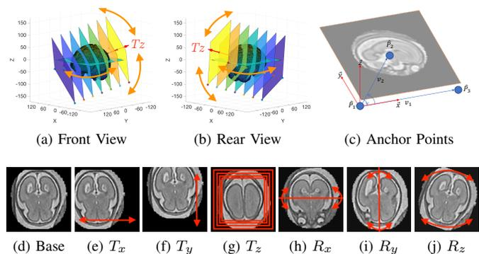
Fig. 2. (a-b) Visualization of extracting  $\omega_i$  from  $\Omega$ . The identity plane lies flat on the  $x-y$  axis, which is then rotated through an Euler Angle Iterator or a Fibonacci Point Iterator and then shifted up and down the normal  $T_z$  (represented by red arrows) to account for out-of-plane transformations. Orange curved arrows represents rotations  $R_x, R_y$  and  $R_z$ . (c) Anchor Point slice parameterization in 3D Space. (d-j) Transformations in 6 DoF.
