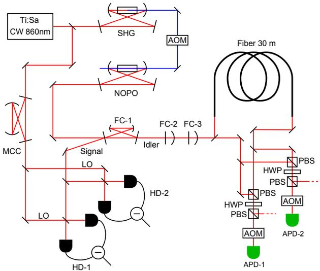
FIG. 5. Experimental setup. Ti:Sa denotes titanium sapphire laser, CW continuous-wave, SHG second harmonic generator, AOM acousto-optic modulator, FC filter cavity, MCC spatial-mode cleaning cavity, LO local oscillator, and HD homodyne detector.
