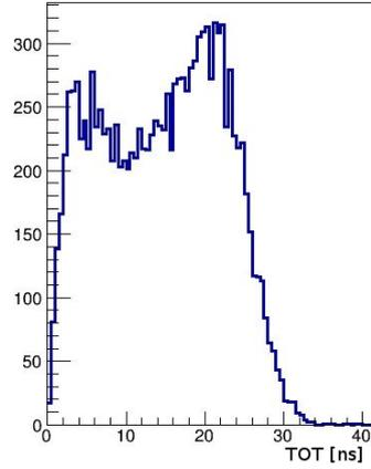
Fig. 5. Distribution of the TOT sum from four thresholds at two photomultipliers connected to the same scintillator. Only back-to-back  $\gamma$  quanta were selected. Test setup consisted of  $^{22}\text{Na}$  source placed inside lead collimator [27]. Source was placed at the center of detection chamber.
