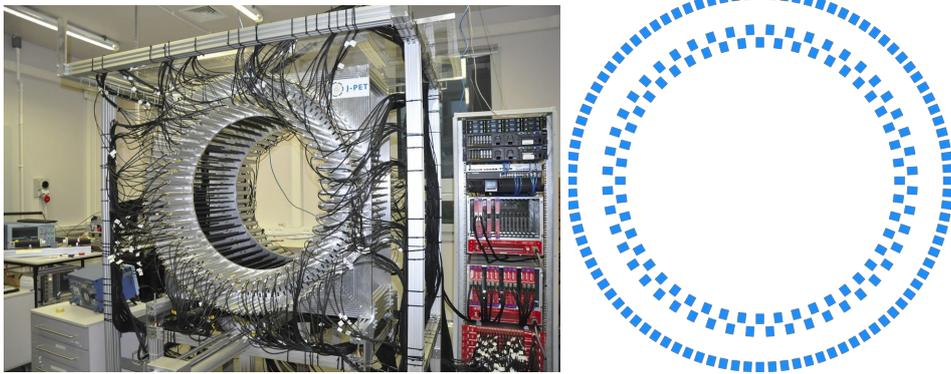
Fig. 4. Photo of the full scale J-PET prototype (left) and layout of detection rings (right). Detection modules are arranged into three non-overlapping rings which cross section is shown schematically on the right panel. Diameters and amount of detection modules from the most internal layer are following: 850 mm and 48, 935 mm and 48, 1150 mm and 96.
