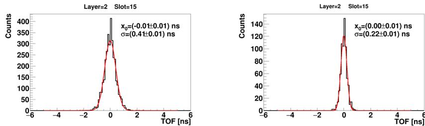
Fig. 7. TOF spectrum for one module from the second layer before- (left) and after (right) the cut on TOT spectrum.  $^{22}\text{Na}$  source was placed inside lead collimator in the center of detection chamber. TOT cut was set to value corresponding to 200 keV of deposited energy.
