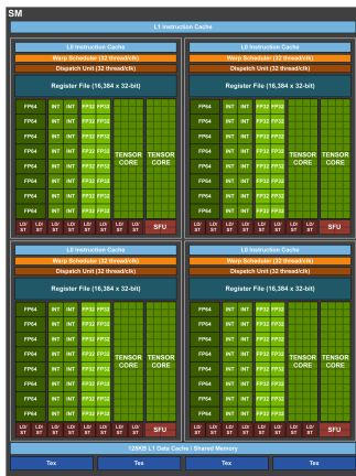
(a) GV100 structure.
