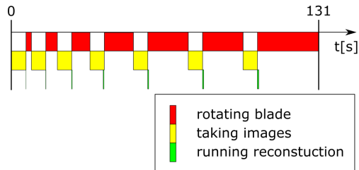
FIGURE 11. Time line of density reconstruction with N_a = 7 projection measurements. The angles are chosen such that more projections are acquired in the direction parallel to the shockfront, maximising the information about the shock. For each projection 20 images were acquired, 10 of which were recorded with the gas jet on and the other 10 with the gas jet off, as a reference.
