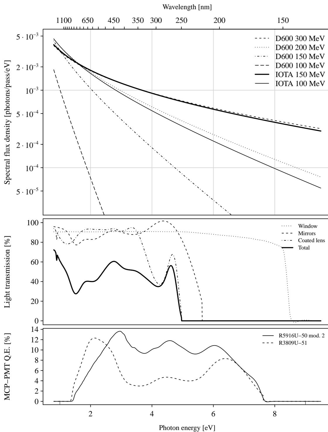
Figure 1. Spectral flux density of synchrotron-light photons (top); transmission of light-transport system (middle); quantum efficiency of photodetector (bottom).
