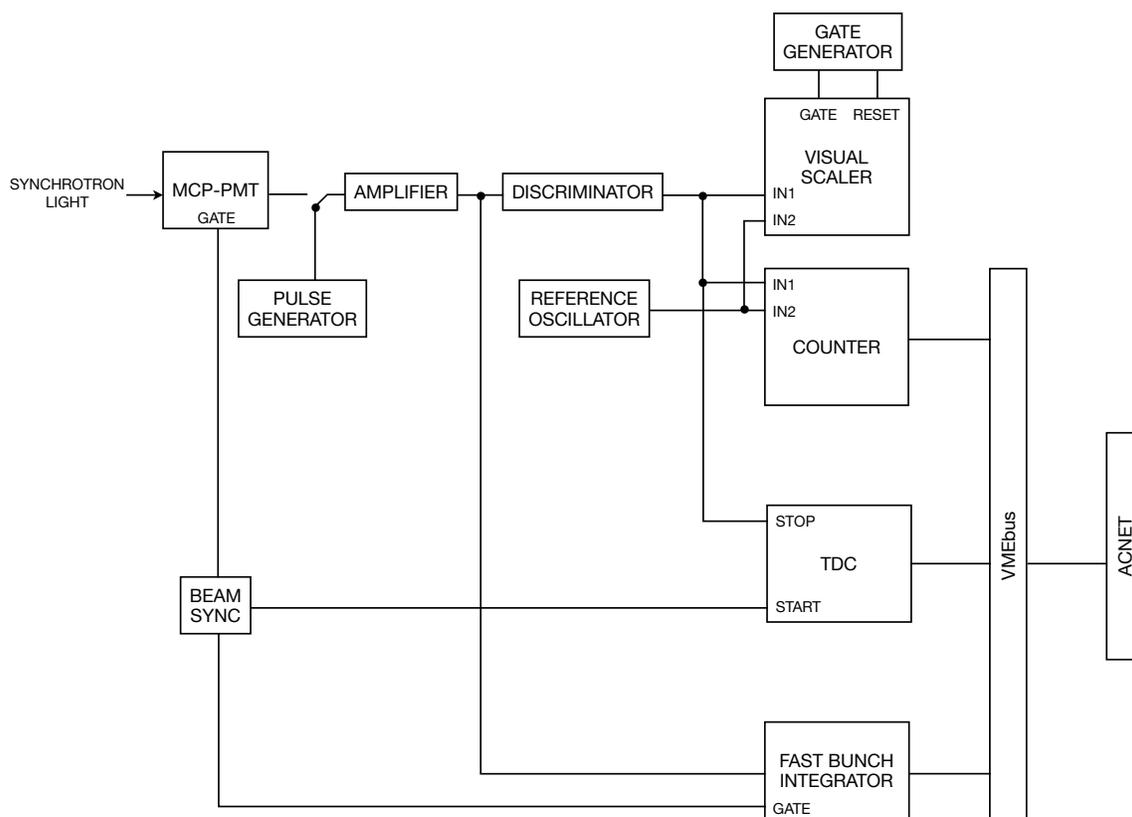
Figure 2. Schematic diagram of the data-acquisition system.
