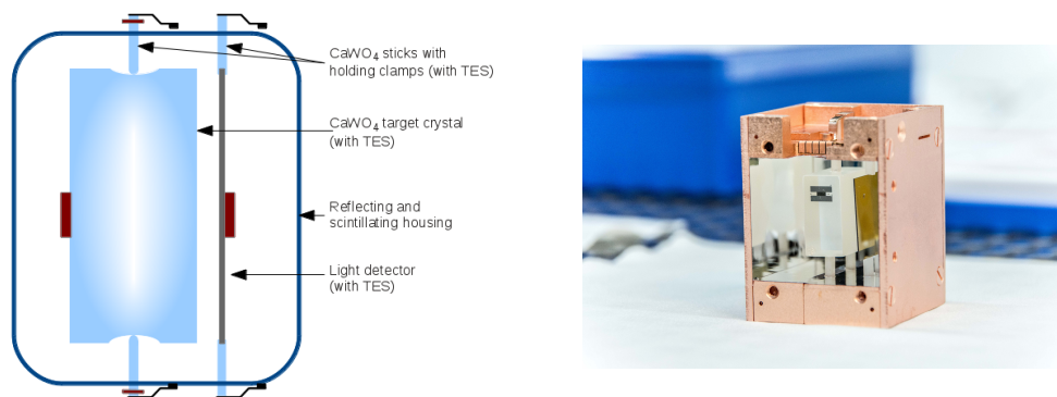
Figure 1. Left: Schematic view of the detector design for CRESST-III modules. Right: Open CRESST-III detector module during mounting in the Gran Sasso facility.
